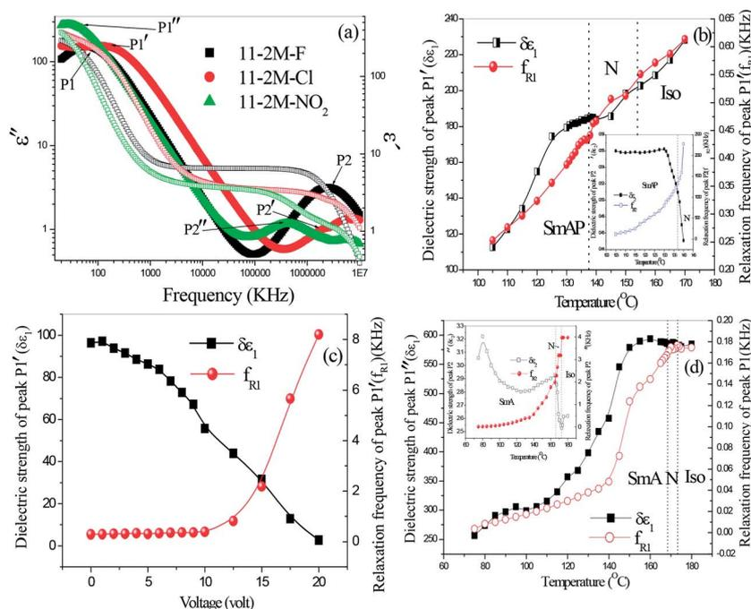
Fig. 4 (a) Dielectric spectra at 130 °C of the compounds 11-2M-F, 11-2M-Cl and 11-2M-NO<sub>2</sub>; (b) temperature dependence of dielectric strength ( $\delta\epsilon$ ) and relaxation frequency ( $f_R$ ) of peak P1' and P2' (inset) of 11-2M-Cl, (c) effect of bias voltage on  $\delta\epsilon$  and  $f_R$  of P1', (d) temperature dependence of dielectric strength ( $\delta\epsilon$ ) and relaxation frequency ( $f_R$ ) of peak P1'' and P2'' (inset) of 11-2M-NO<sub>2</sub>.
