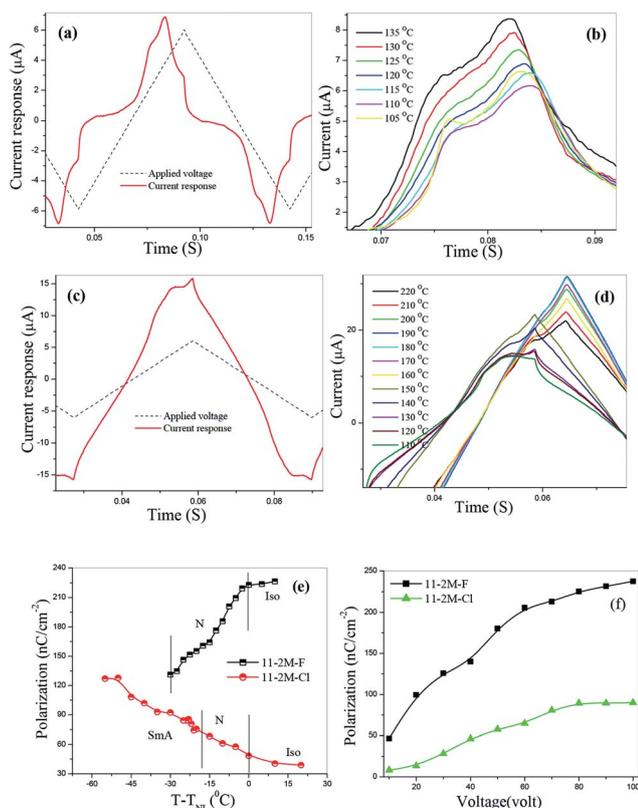
**Fig. 3** Investigation of current response applying triangular wave voltage  $20 V_{PP} \mu m^{-1}$ , 10 Hz for (a) 11-2M-F at  $120^\circ C$ ; (b) 11-2M-F at different temperatures; (c) 11-2M-Cl at  $130^\circ C$ ; (d) 11-2M-Cl at different temperatures; (e) temperature dependence of spontaneous polarization for 11-2M-F and 11-2M-Cl and (f) voltage variation of spontaneous polarization for 11-2M-F and 11-2M-Cl.
