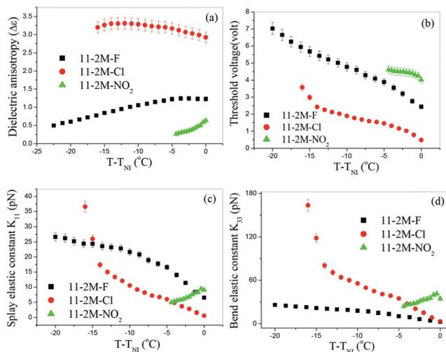
**Fig. 2** Variation of (a) dielectric anisotropy ( $\Delta\epsilon = \epsilon_{\parallel} - \epsilon_{\perp}$ ), (b) threshold voltage ( $V_{th}$ ), (c) splay elastic constant ( $K_{11}$ ) and (d) bend ( $K_{33}$ ) elastic constant as a function of reduced temperature ( $T - T_{NI}$ ). The error bar corresponds to 5% experimental error.
