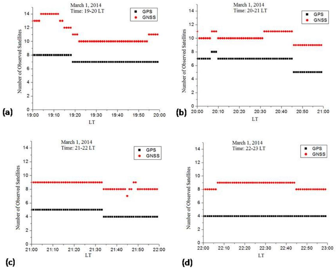
Figure 6: Number of GPS and GNSS satellites tracked every hour during 19:00-23:00LT on March 1, 2014 from Calcutta. The red dots indicate the number of multi-constellation satellites, combining GPS, GLONASS and GALILEO, while the black dots represent the number of GPS satellites.
