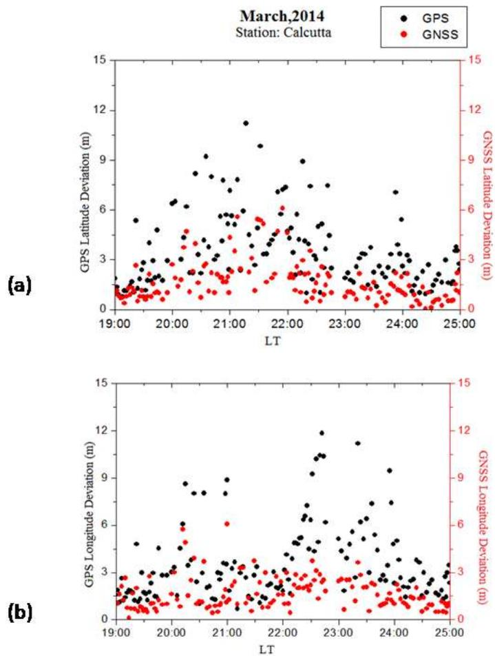
Figure 8: Composite plot for the month of March 2014 showing 99 percentile position errors of the receiver (a) latitude and (b) longitude, expressed in metres, during 19:00-01:00LT of different days. The black points show GPS positioning errors while the red ones indicate GNSS positioning errors.
