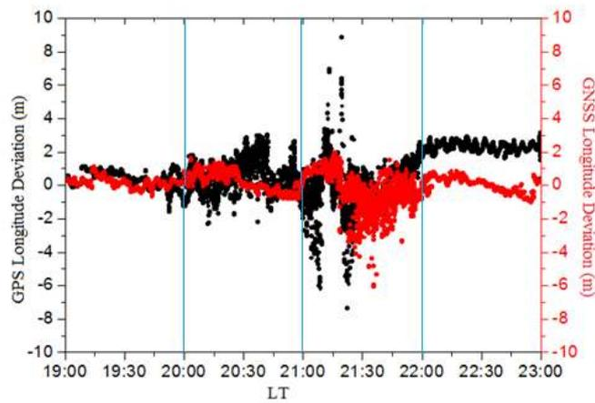
Figure 7: Receiver (a) latitude and (b) longitude deviations when using GPS and multi-constellation measured in meters during 19:00-23:00LT on March 1, 2014 at Calcutta. The black points correspond to GPS while the red ones indicate GNSS.
