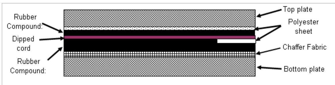
Fig 2. Layers of rubber compound and tyre cord
