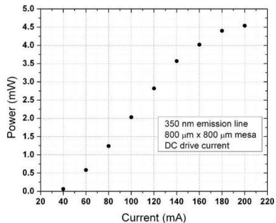
FIG. 7. Integrated power output of an UV-LED device with a peak intensity at 350 nm under dc operation vs drive current.
