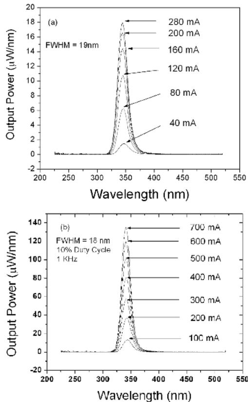
FIG. 4. Electroluminescence spectra, plotted as output power/nanometer vs wavelength, of an UV-LED device with a peak intensity at 340 nm under (a) dc and (b) pulsed operations at various drive currents.
