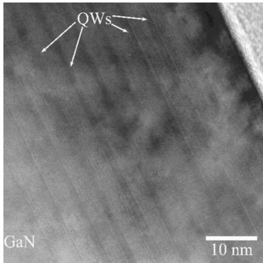
FIG. 2. HRTEM image of GaN/Al<sub>0.2</sub>Ga<sub>0.8</sub>N MQWs consisting of barriers having 16 monolayers, and wells having 6 monolayers, viewed along the [1 $\bar{1}$ 00] direction.
