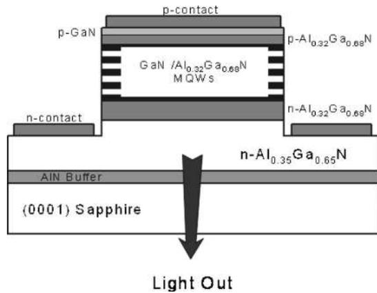
FIG. 1. Schematic illustration of the investigated UV-LED structures showing the various device layers.
