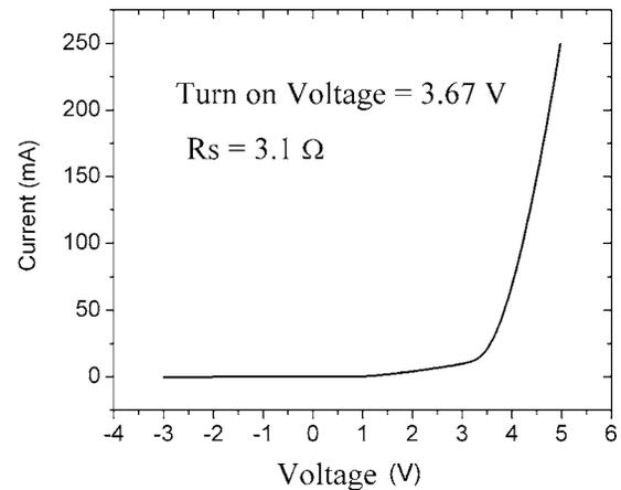
FIG. 3. *I*-*V* characteristics of an UV-LED device emitting at 340 nm. Indicated in the inset of the figure are the turn-on voltage and on-series resistance of the device.
