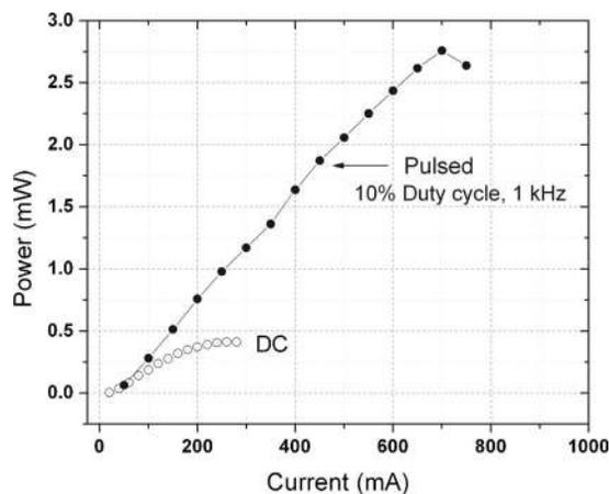
FIG. 5. Integrated power output of an UV-LED device with a peak intensity at 340 nm under dc and pulsed operations vs drive current.
