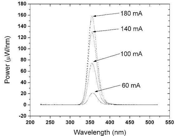
FIG. 6. Electroluminescence spectra, plotted as output power/nanometer vs wavelength, of an UV-LED device with a peak intensity at 350 nm under dc operation at various drive currents.
