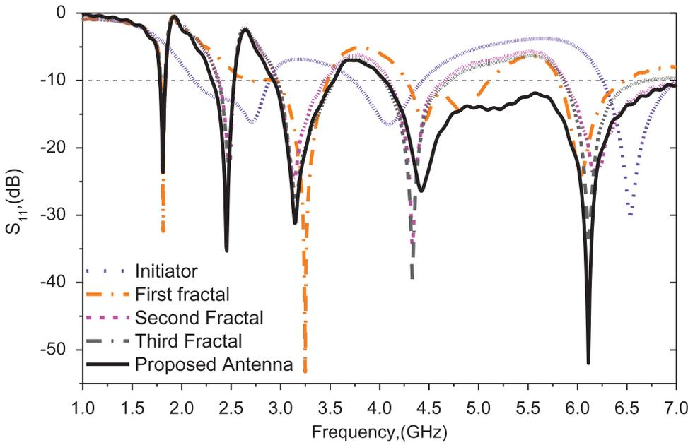
Figure 3: Simulated  $S_{11}$  of antenna for various design steps as shown in Figure 2 (a)-(e)..
