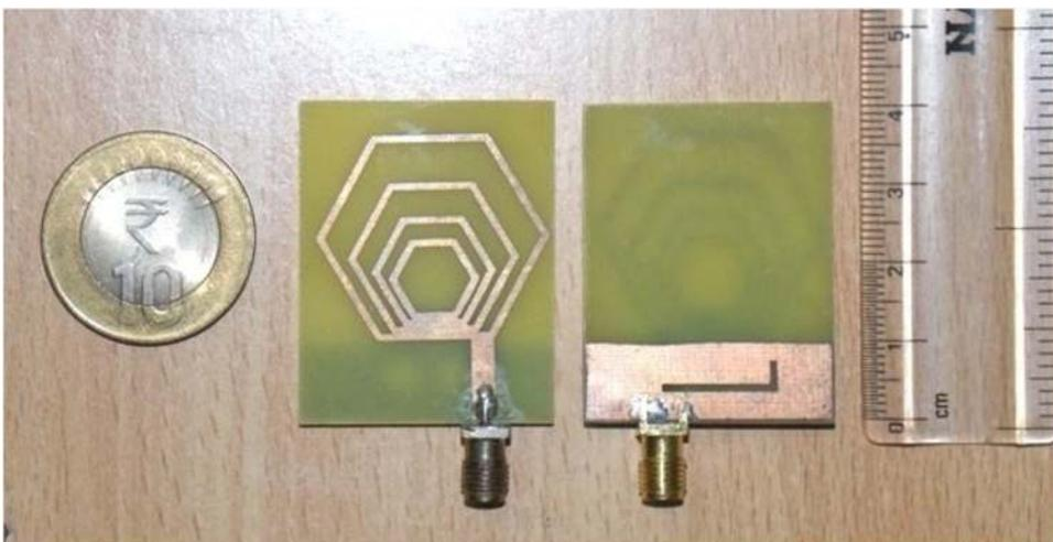
Figure 5: Photograph of the fabricated antenna.
