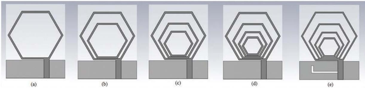
Figure 2: Design steps of proposed antenna (a) Initiator (b) First Fractal (c) Second Fractal (d) Third fractal (e) Proposed design.
