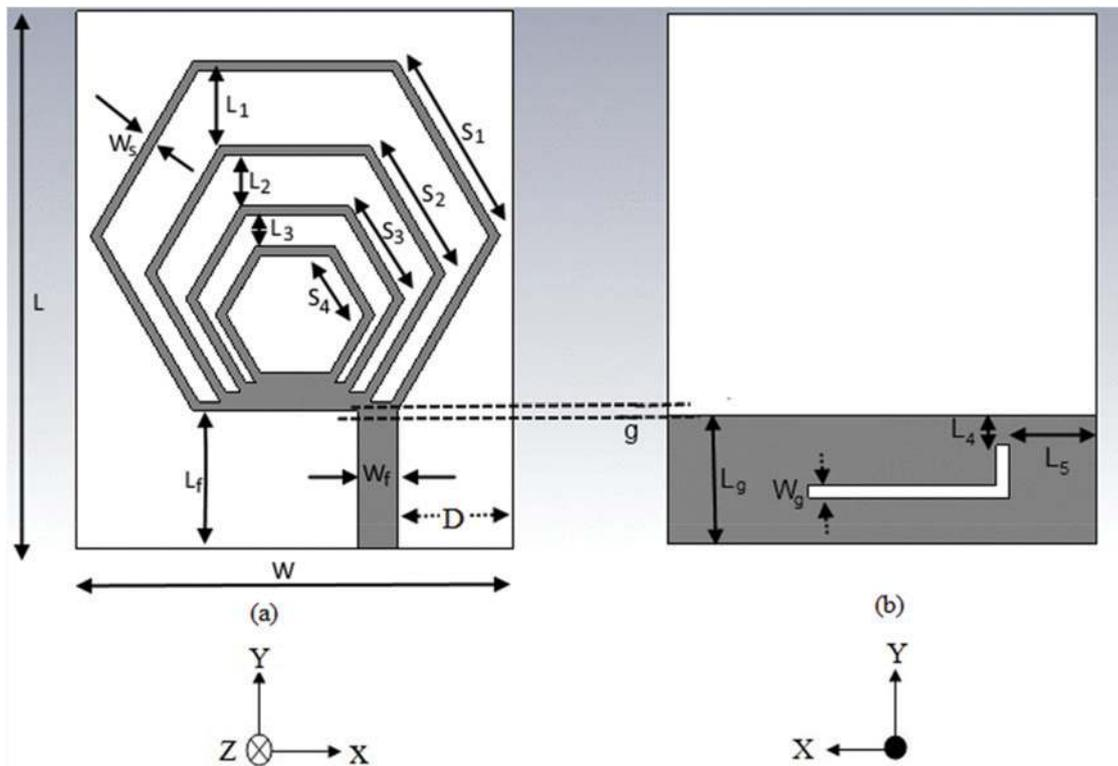
Figure 1: Proposed antenna (a) front view (b) back view.
