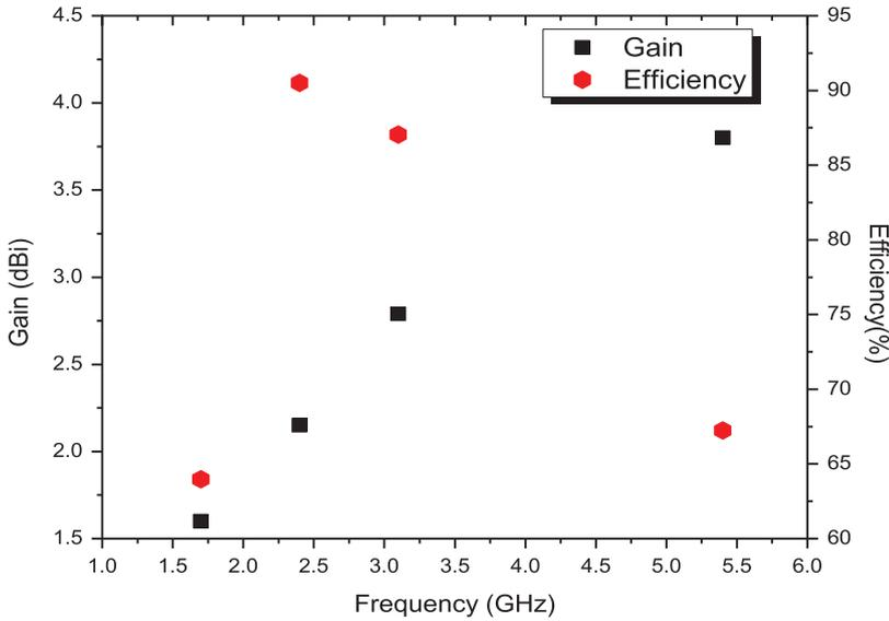
Figure 10: Measured Gain and Simulated Efficiency of proposed antenna.
