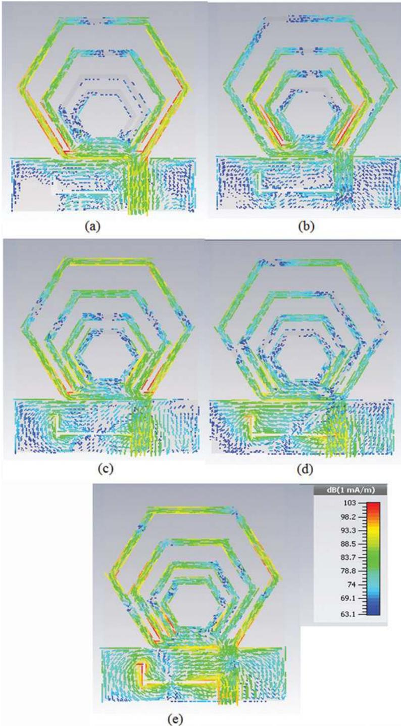
**Figure 8:** Simulated surface current distributions on the radiating patch of proposed antenna at (a) 1.7 GHz (b) 2.4 GHz (c) 3.1 GHz (d) 4.5 GHz (e) 6 GHz.
