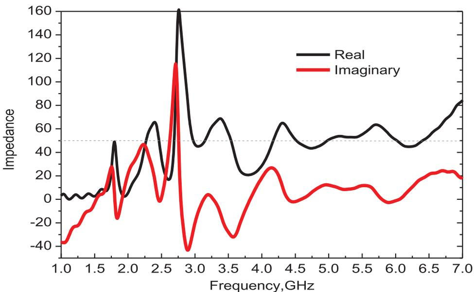
Figure 7: Simulated real and imaginary impedance of the proposed antenna.
