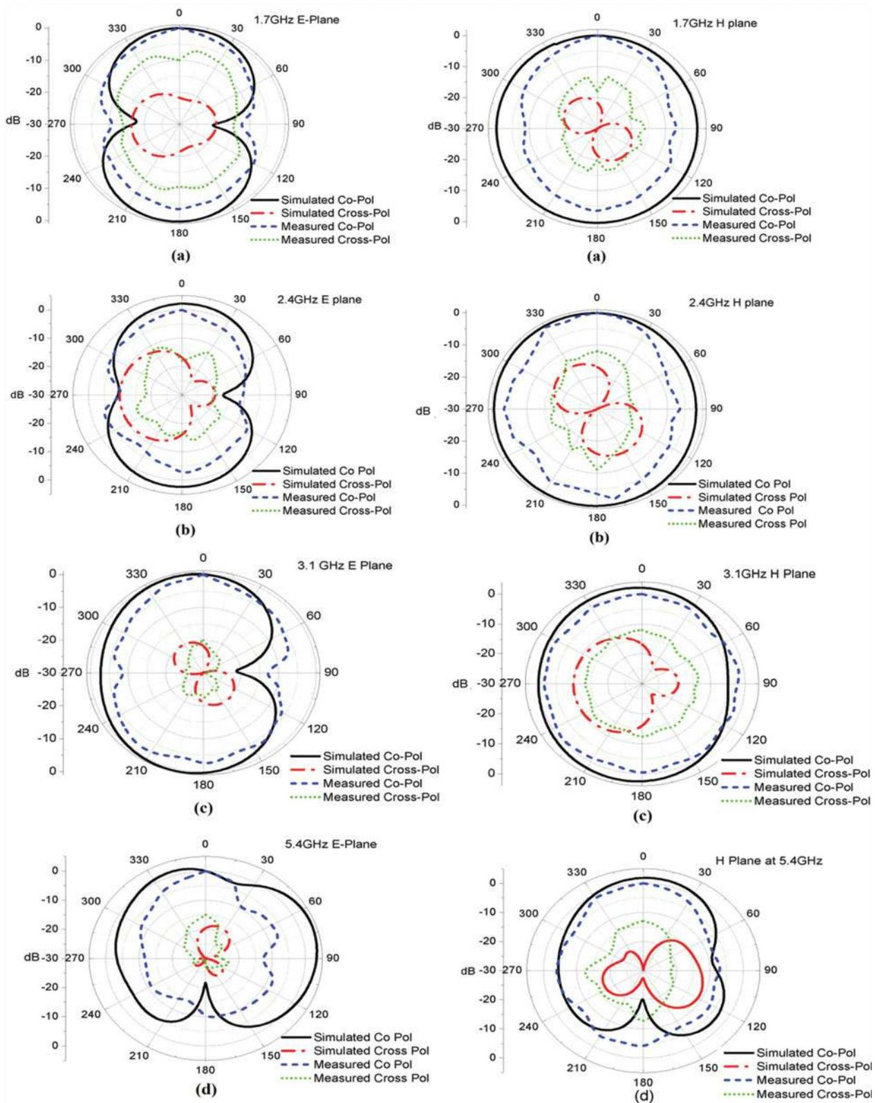
Figure 9: Simulated and Measured Co and Cross Pol of proposed antenna in E(yz plane) and H(xz-plane) planes at (a) 1.7 GHz (b) 2.4 GHz (c) 3.1 GHz (d) 5.4 GHz.
