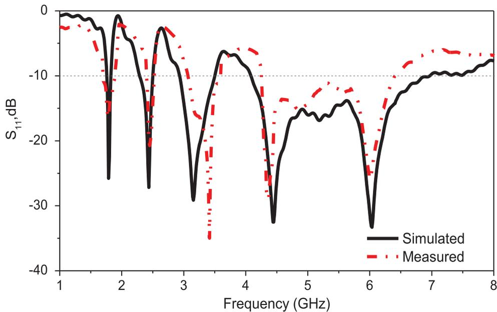
Figure 6: Measured and Simulated  $S_{11}$  for proposed design antenna at 1.7 GHz, 2.4 GHz, 3.1 GHz, 4.5 GHz and 6.0 GHz.
