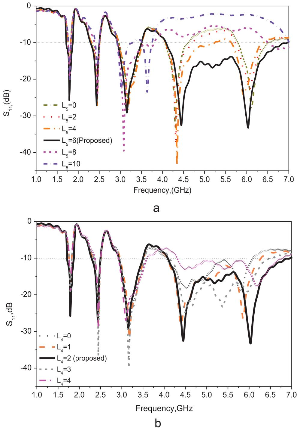
**Figure 4:** (a) Effect of slot position along x-axis (horizontal movement) with respect to different value of  $L_5$  on ground plane for  $L_4 = 2$  mm (constant) as shown in Figure 1(b). (b) Effect of slot position along y axis (vertical movement) with respect to different value of  $L_4$  on ground plane for  $L_5 = 6$  mm (constant) as shown in Figure 1(b).
