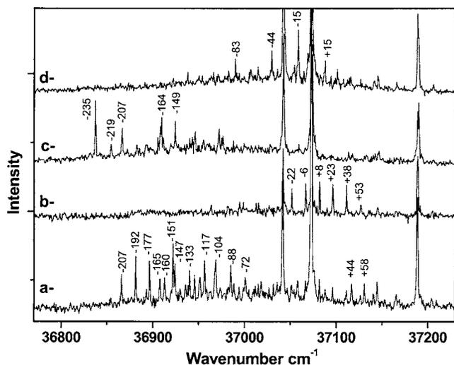
FIG. 7. Laser-induced fluorescence (LIF) excitation spectrum of jet-cooled (*R*)-indan-1-ol with (a) (*S*)-methyl-lactate and (b) (*R*)-methyl-lactate and (*R*)-indan-1-ol with (c) (*S*)-ethyl-lactate and (d) (*R*)-ethyl-lactate.
