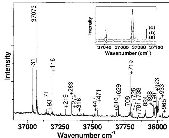
FIG. 1. Laser-induced fluorescence (LIF) excitation spectrum of jet-cooled indan-1-ol in the band origin region. Inset: Excitation spectra at three different sample temperatures: (a) 25 °C, (b) 40 °C, and (c) 60 °C.
