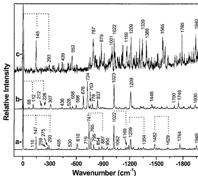
FIG. 2. Single vibronic level emission spectra of indan-1-ol excited at (a)  $37\,073\text{ cm}^{-1}$  (band A), (b)  $37\,042\text{ cm}^{-1}$  (band B), and (c)  $37\,144\text{ cm}^{-1}$  (band C).
