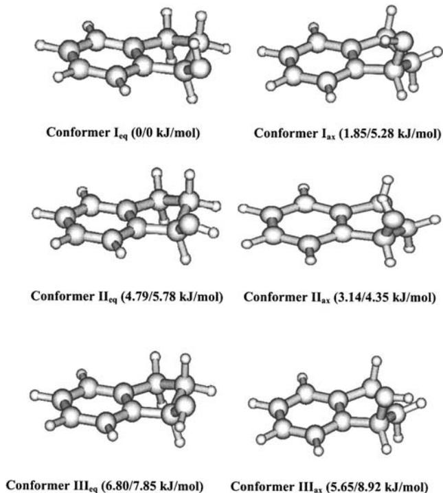
FIG. 5. Calculated low-energy conformers of indan-1-ol for the ground state at the MP2 level with 6-31G\*\* basis set. The numbers in parentheses are the relative energies (first value from MP2 and second value from DFT calculations) with respect to the minimum energy structure.
