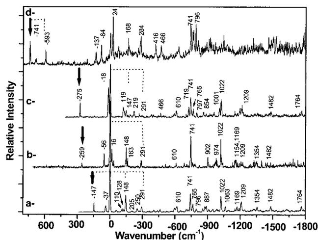
FIG. 3. Single vibronic level emission spectra of indan-1-ol excited at (a) 37 073+116 cm<sup>-1</sup>, (b) 37 073+219 cm<sup>-1</sup>, (c) 37 073+263 cm<sup>-1</sup>, and (d) 37 073+719 cm<sup>-1</sup> bands. The zero of the scale is set on the 37 073 cm<sup>-1</sup> transition. The arrow shows the excitation wavelength.
