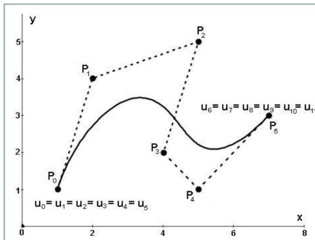
Figure 4 B-spline curve of the degree  $k = 5$
