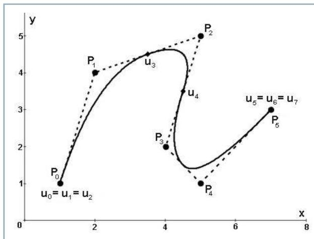
Figure 6 B-spline curve of the degree  $k = 2$
