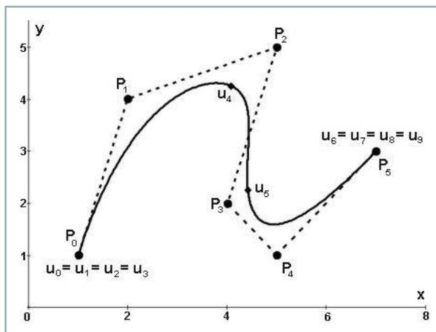
Figure 5 5 B-spline curve of the degree  $k = 3$
