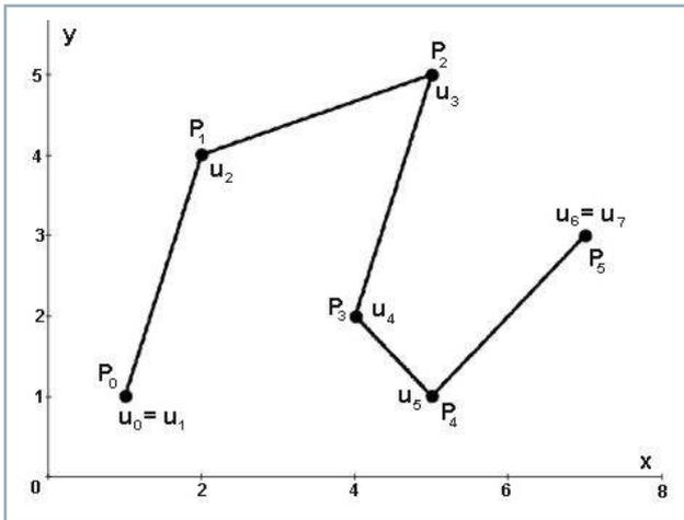
Figure 7 B-spline curve of the degree  $k = 1$
