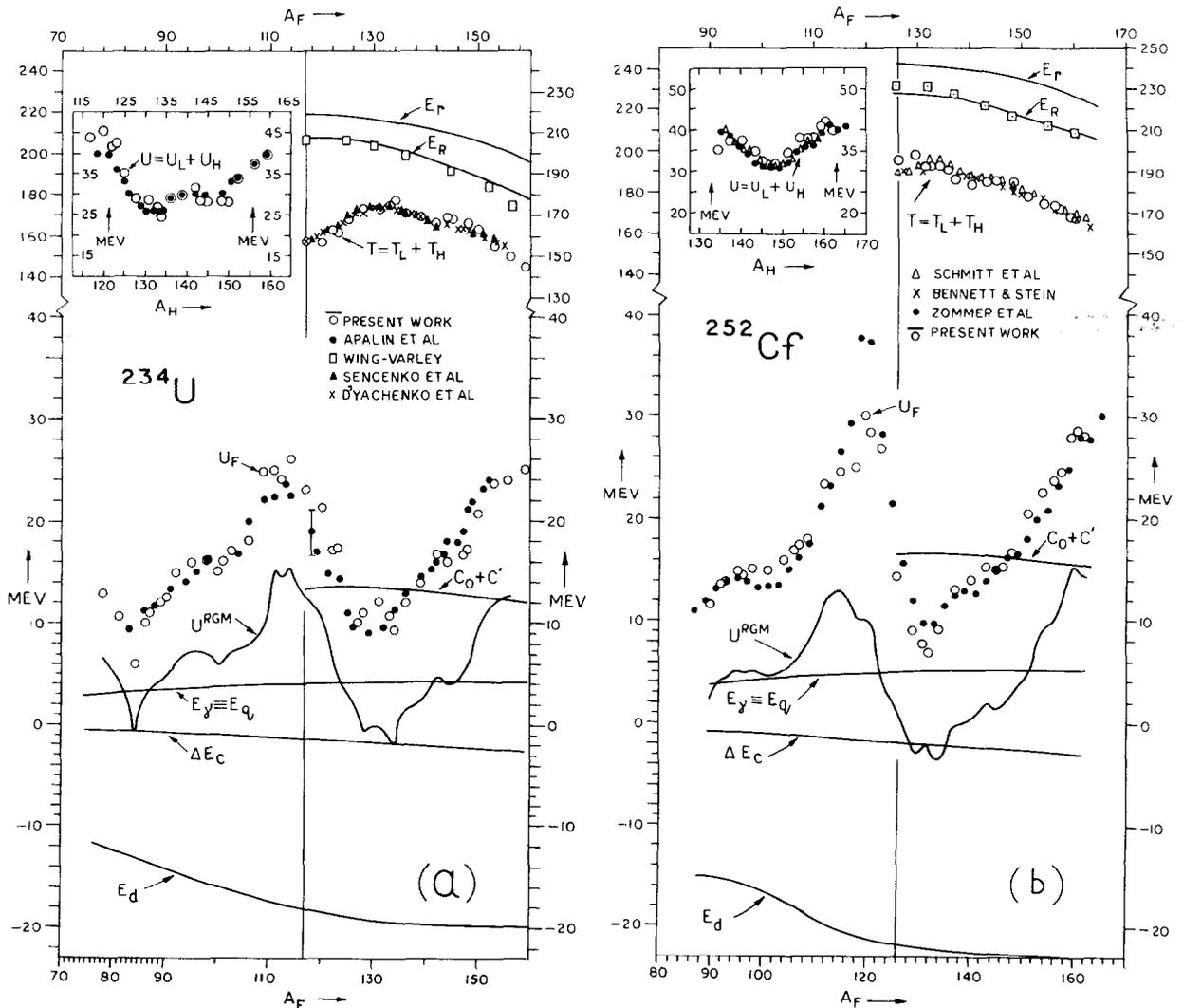
Fig. 2. The energies in the fission processes of a) the thermal neutron induced fission of  $^{233}\text{U}$  and b) the spontaneous fission of  $^{252}\text{Cf}$ . See text for the origin of various energy terms. Note that the total energy release  $E_R$ , the fragment excitation  $U_F$ , the total excitation  $U = U_L + U_H$  in the inserts at left, and the total kinetic energy  $T$  agree with observations fairly satisfactorily in both cases.
