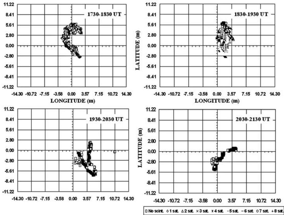
**Figure 4.** Position deviations of Calcutta observed with GPS during 1730–2130 UT (2330–0330 LT) on 12 February 2001. The legend shows the number of satellites simultaneously exhibiting scintillations in excess of 10 dB corresponding to each position value.
