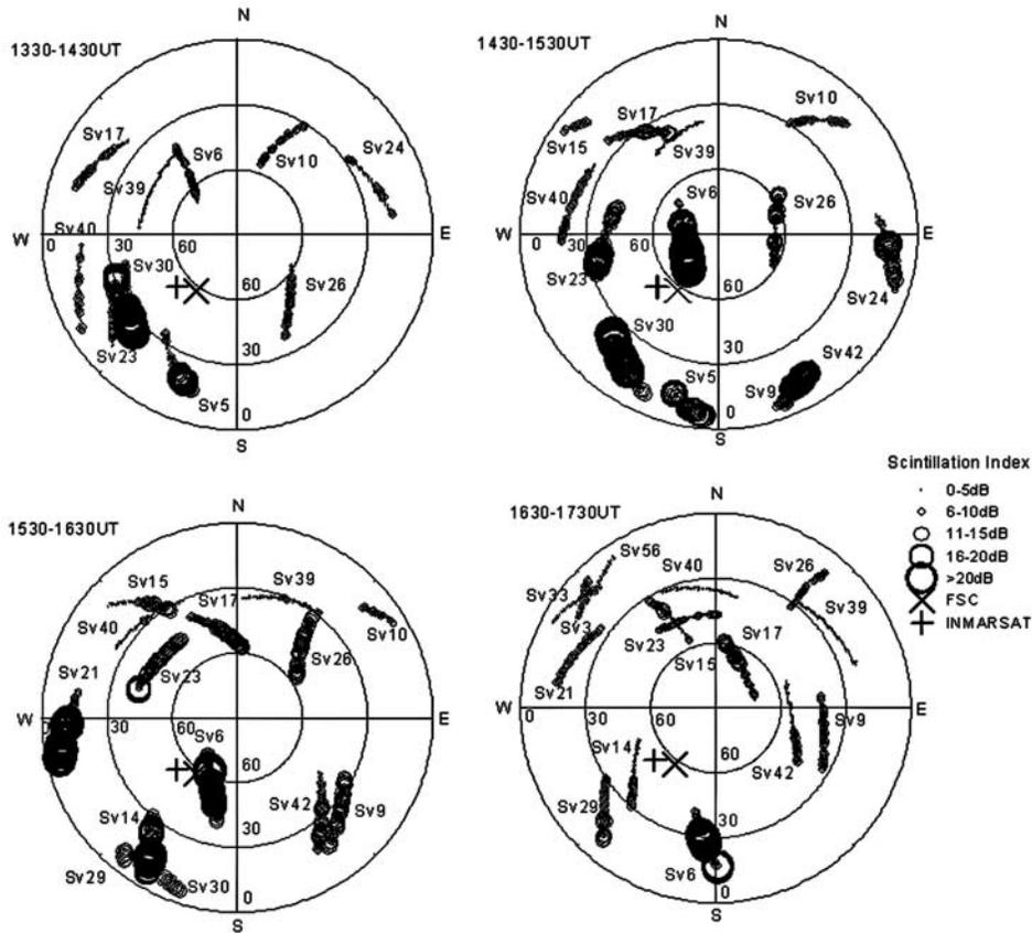
**Figure 1.** Elevation-azimuth plots of GPS satellite tracks observed from Calcutta during 1330–1730 UT (1930–2330 LT) on 12 February 2001. The superimposed circles show the observed scintillation index (SI) (in decibels).
