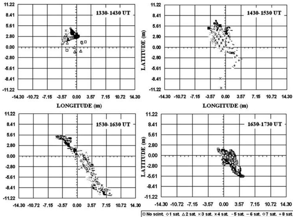
**Figure 3.** Position deviations of Calcutta observed with GPS during 1330–1730 UT (1930–2330 LT) on 12 February 2001. The legend shows the number of satellites simultaneously exhibiting scintillations in excess of 10 dB corresponding to each position value.
