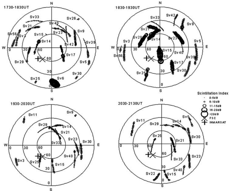
**Figure 2.** Elevation-azimuth plots of GPS satellite tracks observed from Calcutta during 1730–2130 UT (2330–0330 LT) on 12 February 2001. The superimposed circles show the observed SI (in decibels).
