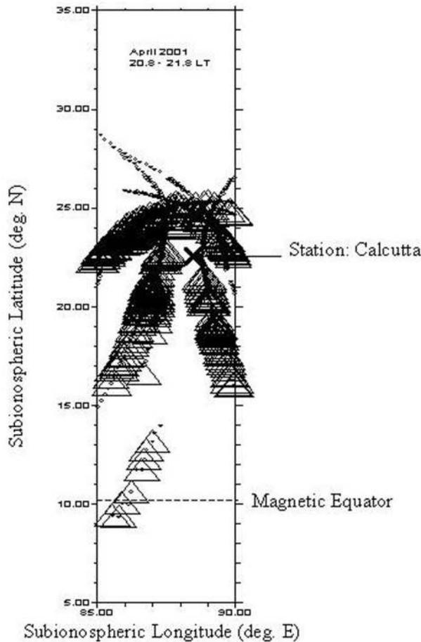
**Figure 5.** Plot of 350-km subionospheric tracks of GPS satellites observed from Calcutta during 2048–2148 LT in April 2001. The triangles represent points on the track with scintillations in excess of 15 dB, and the dots represent points with no scintillations. The position of the station is indicated by the cross. Observations had been limited to a  $5^\circ$  longitude swath about the station. The traces are smudged because of overlapping of several GPS passes observed over 1 month.
