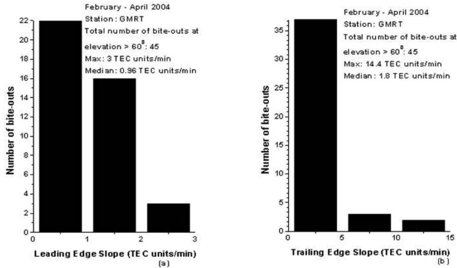
**Figure 9.** (a) Distribution of leading (eastern wall of the irregularity) edge of the bite-out in TEC observed from the GMRT site along the tracks of different GPS satellites during February–April 2004 at elevation angles exceeding 60°. (b) Distribution of trailing (western wall of the irregularity) edge of the bite-out in TEC observed from the GMRT site along the tracks of different GPS satellites during February–April 2004 at elevation angles exceeding 60°.
