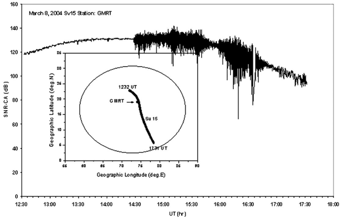
**Figure 4.** SNR-CA for SV15 plotted against universal time observed from the GMRT site on 8 March 2004. The inset shows the track of the same satellite with the start and end time. The ellipse indicates the zone of reception at  $5^\circ$  mask angle.
