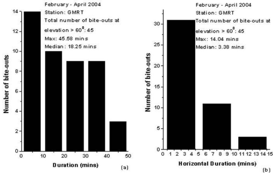
**Figure 8.** (a) Distribution of duration of bite-outs in TEC along the tracks of different GPS satellites observed from the GMRT site during February–April 2004 when the elevation angle is greater than 60°. (b) Distribution of west-east duration of bite-outs in TEC taking into account the projected inclination of the GPS orbits at the ionospheric height of 350 km.
