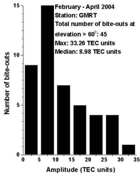
**Figure 7.** Amplitude distribution of TEC depletions observed from the GMRT site along the tracks of different GPS satellites during February–April 2004 at elevation angles exceeding  $60^\circ$ .
