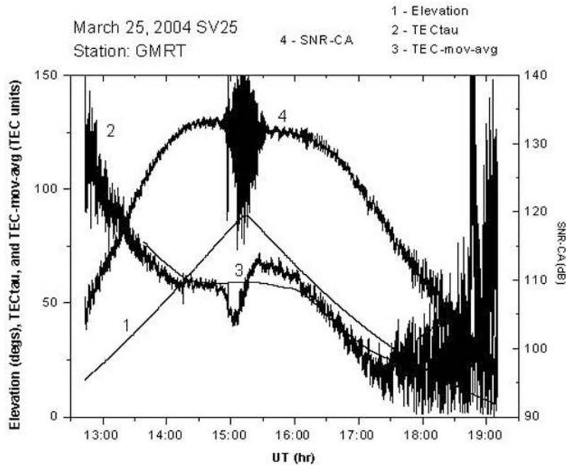
**Figure 2.** Typical sample record from GPS satellite SV25 observed from the GMRT site on 25 March 2004. Curve 1 refers to the elevation angle of the satellite during its transit, curve 2 represents the total electron content (TEC) calculated from the group delay (TECtau), curve 3 is the 90-min moving-averaged TECtau (TEC-mov-avg), and curve 4 shows the signal-to-noise ratio for the satellite link operated in the coarse acquisition (C/A) mode (SNR-CA).
