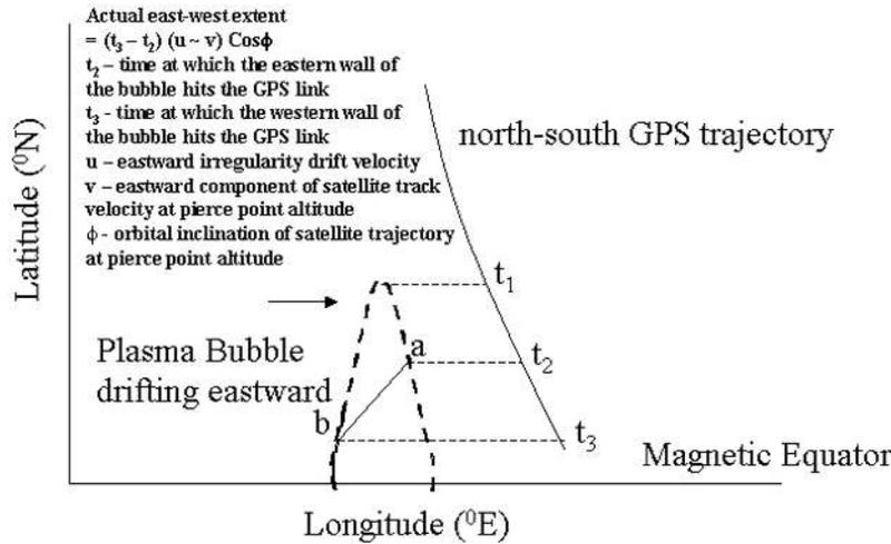
**Figure 1.** Sketch of a typical equatorial plasma bubble, which is wide over the magnetic equator and narrows down north of the station, drifting eastward. A north-south GPS trajectory is intercepted by the bubble during the time interval  $(t_3 - t_2)$ , where  $t_2$  corresponds to the time when the eastern wall of the bubble hits the GPS link, and  $t_3$  corresponds to the time when the western wall hits the link. Section  $ab$  is the apparent spatial extent of the bubble.
