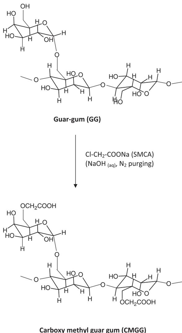
Fig. 1. Derivatization scheme of guar gum by carboxymethylation.
