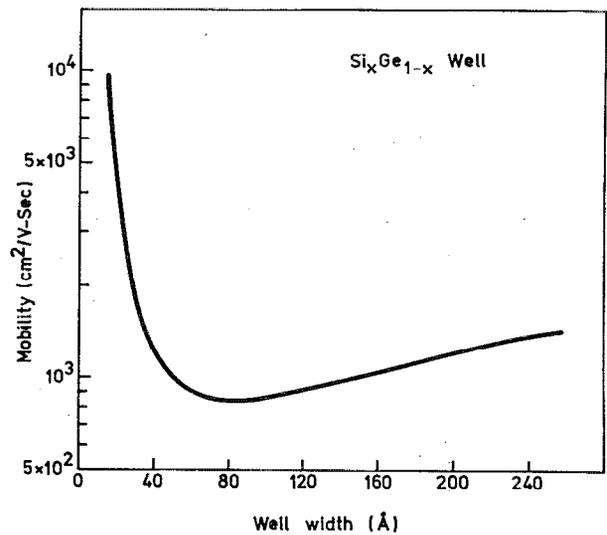
FIG. 2. Dependence of the alloy-disorder scattering limited electron mobility on the width of the quantum well. The electrons are assumed to be confined in the Si<sub>0.5</sub>Ge<sub>0.5</sub> layer.
