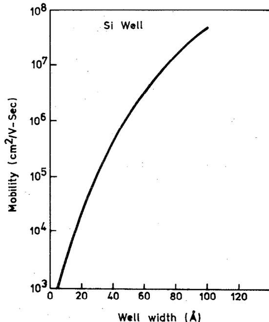
FIG. 3. Dependence of the alloy-disorder scattering limited electron mobility on the width of the quantum well. The electrons are assumed to be confined in the Si layer.
