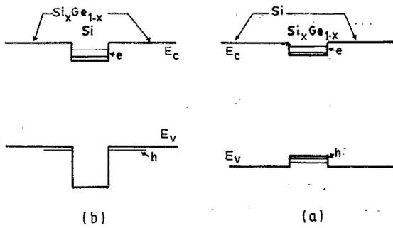
FIG. 1. Band diagrams for a Si-Si<sub>x</sub>Ge<sub>1-x</sub> QW: (a) type-I and (b) type-II alignment.  $E_{c(v)}$  refers to the conduction-(valence) band edge.
