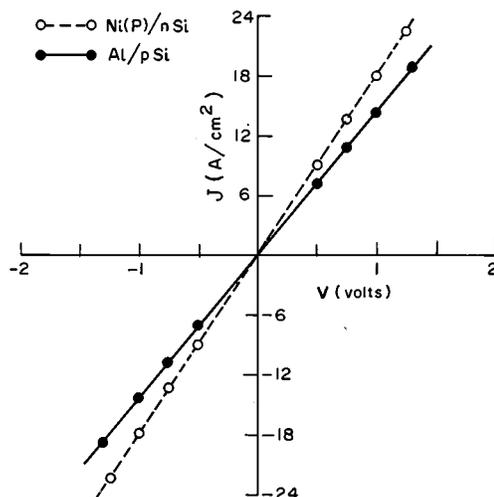
FIG. 3. Current–voltage characteristics of electroless Ni(P) and evaporated Al contacts on polished *n*- and *p*-type Si surfaces, respectively.
