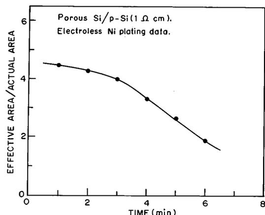
FIG. 1. Effective area of Ni plating on PSi, shown as a function of the plating time.
