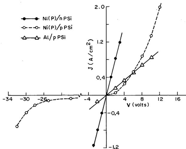
FIG. 2. Current–voltage characteristics of electroless Ni(P) and evaporated Al contacts on PSi.
