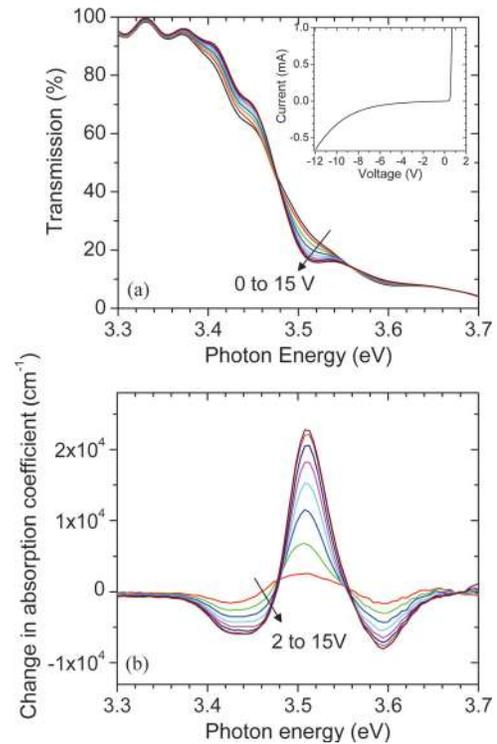
FIG. 5. (Color online) (a) Normalized transmission spectra through a GaN/AlGaN multiple-QW modulator for different values of the applied reverse bias voltage (0, 2, 4, 6, 8, 10, 12, 14, and 15 V). The inset shows the current-voltage characteristics of the same device. (b) Differential absorption spectra derived from the traces of (a).
