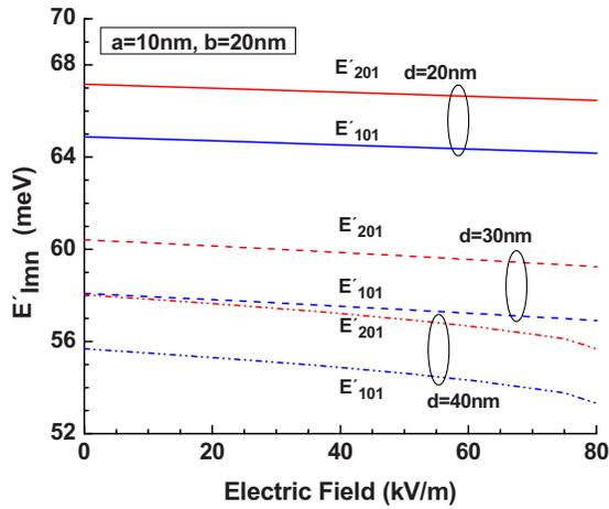
FIG. 3. (Color online) Two lowest energy states of electrons in a cylindrical quantum ring as a function of electric field for  $a=10$  nm,  $b=20$  nm, and three different values of thickness,  $d=20, 30,$  and  $40$  nm.
