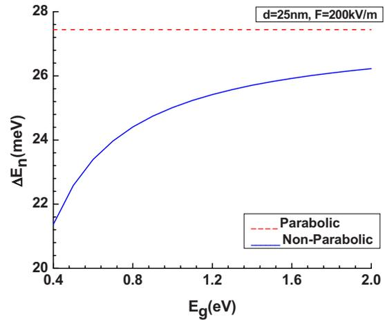
FIG. 5. (Color online) Transition energy between two lowest subbands  $\Delta E_n$  (i.e.,  $\Delta E_1 = E'_{102} - E'_{101}$ ) plotted as a function of band gap,  $E_g$ , for  $F=200$  kV/m and  $d=25$  nm. The dashed straight line indicates the result obtained using assumption of parabolicity of band.
