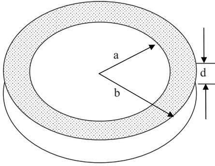
FIG. 1. Schematic structure of a cylindrical quantum ring. The inner and outer radii are  $a$  and  $b$ , respectively. The thickness of the ring is  $d$ .
