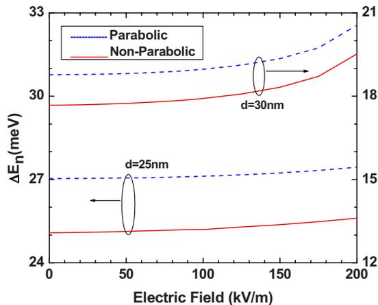
FIG. 4. (Color online) Transition energy between two lowest subbands  $\Delta E_n$  (i.e.,  $\Delta E_1 = E'_{102} - E'_{101}$ ) plotted as a function of electric field ranging from  $F=0$  kV/m to 200 kV/m, taking  $E_g=1.0$  eV for two values of thickness,  $d=25$  and  $30$  nm. The dashed lines show the results with parabolic assumption of the band structure.
