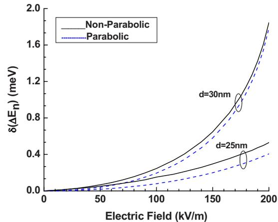
FIG. 6. (Color online) The range of tuning for intersubband transition,  $\delta(\Delta E_1)$ , between two lowest subbands for transition ( $E'_{102} \leftarrow E'_{101}$ ) as a function of electric field taking  $E_g=1.0$  eV for two different values of ring thicknesses ( $d=25$  and  $30$  nm). The dashed lines show the results with the assumption of band parabolicity.
