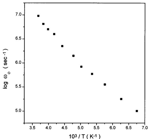
FIG. 7. The logarithm of  $\omega_0$  is plotted as a function of inverse temperature for specimen No. 3.
