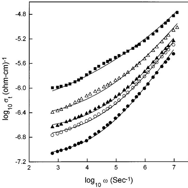
FIG. 4. Variation of ac conductivity as a function of frequency for specimen No. 1 at different temperatures; (■) 306.5 K, (△) 266.8 K, (▲) 244.7 K, (○) 238.5 K, and (●) 217.3 K.
