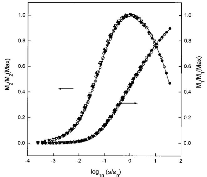
FIG. 6. Real and imaginary parts of dielectric modulus as a function of frequency for specimen No. 3; (▼) 251.0 K, (▲) 239.7 K, (□) 225.9 K, (▽) 209.4 K, (○) 186.6 K, (●) 173.6 K.
