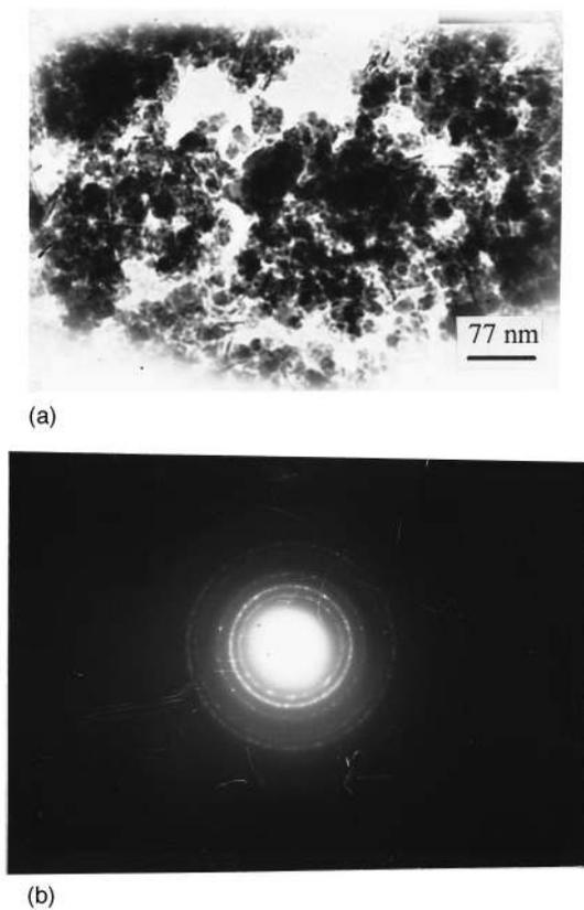
FIG. 1. (a) Transmission electron micrograph for specimen No. 1; (b) electron diffraction pattern obtained from (a).
