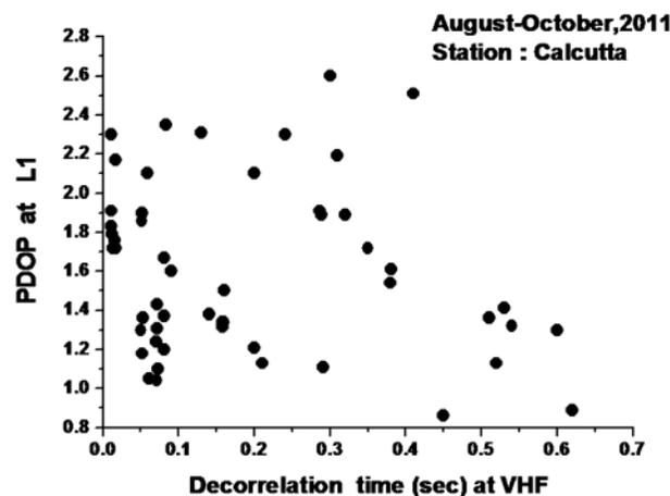
**Figure 7.** Correlation of Position Dilution of Precision (PDOP) for GPS with ionospheric irregularity decorrelation time at VHF (250 MHz) measured from Calcutta during August through October 2011.
