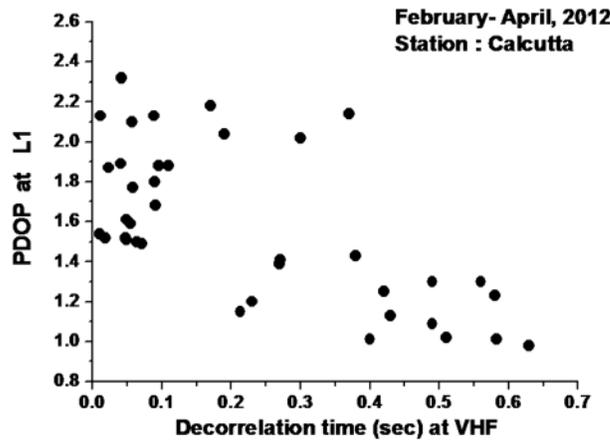
**Figure 8.** Correlation of Position Dilution of Precision (PDOP) for GPS with ionospheric irregularity decorrelation time at VHF (250 MHz) measured from Calcutta during February through April 2012.
