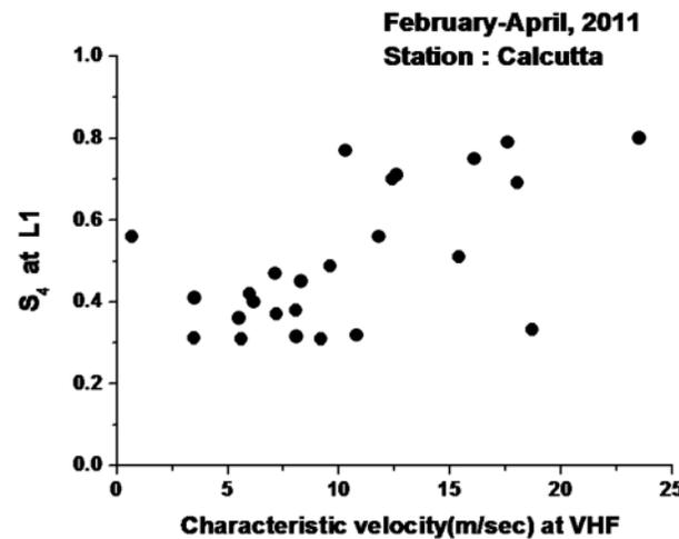
**Figure 3.** Variation of amplitude scintillation index  $S_4$  at GPS L1 frequency with ionospheric irregularity characteristic velocity at VHF (250 MHz) measured from Calcutta during February through April 2011.
