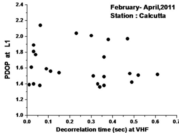
**Figure 6.** Correlation of Position Dilution of Precision (PDOP) for GPS with ionospheric irregularity decorrelation time at VHF (250 MHz) measured from Calcutta during February through April 2011.
