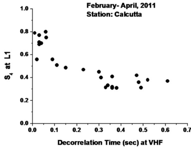
**Figure 4.** Variation of amplitude scintillation index  $S_4$  at GPS L1 frequency with ionospheric irregularity decorrelation time at VHF (250 MHz) measured from Calcutta during February through April 2011.
