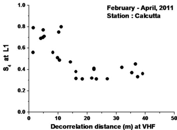
**Figure 5.** Variation of amplitude scintillation index  $S_4$  at GPS L1 frequency with ionospheric irregularity decorrelation distances at VHF (250 MHz) measured from Calcutta during February through April 2011.
