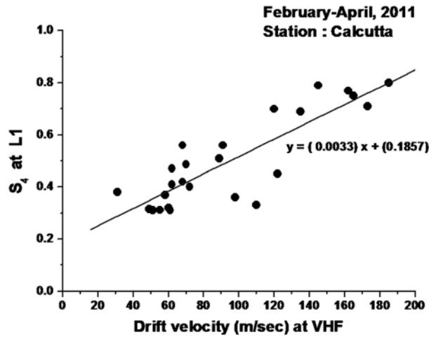
**Figure 2.** Variation of amplitude scintillation index  $S_4$  at GPS L1 frequency with ionospheric irregularity drift velocity at VHF (250 MHz) measured from Calcutta during February through April 2011.
