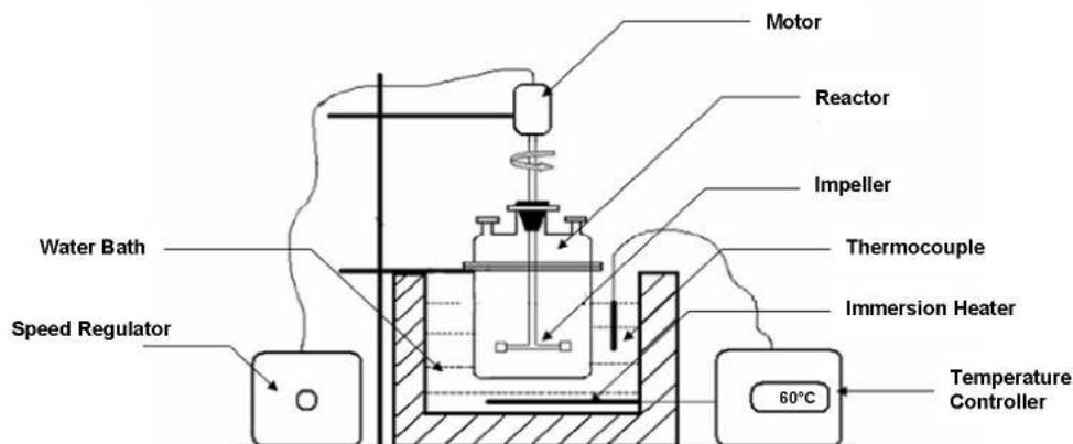
**Figure 1:** Schematic diagram of the experimental set up.
