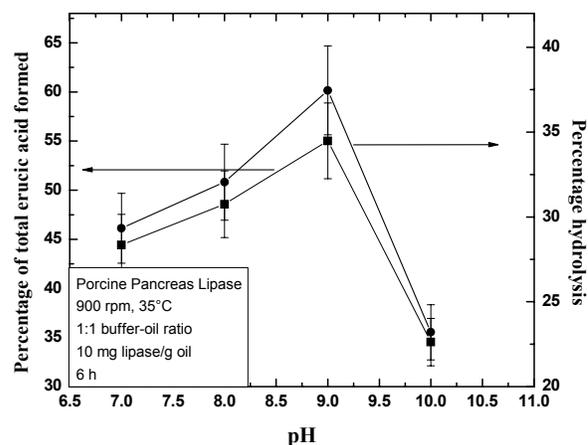
**Figure 3:** Variation of 'percentage of total erucic acid formed' and 'percentage hydrolysis' with pH.
