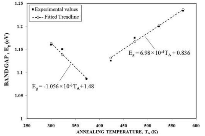
FIG. 7. The variation of the band gap energy with the annealing temperature.
