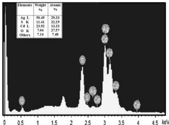
FIG. 2. The EDS results of as-deposited  $\text{Ag}_2\text{S}$  thin film prepared by chemical conversion method.
