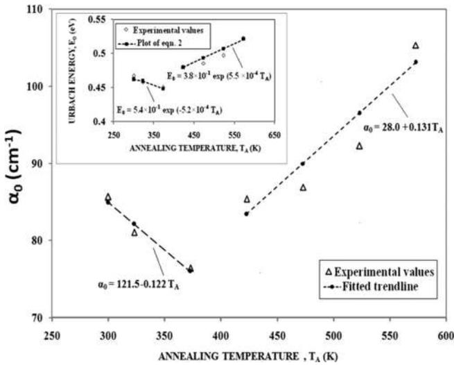
FIG. 5. Dependence of Urbach parameters,  $\alpha_0$  and  $E_0$ , on the temperature of annealing,  $T_A$ . Dashed line curves represent linearly fitted relations describing the experimental values of  $\alpha_0$ . The inset shows the variation of Urbach energy,  $E_0$  with annealing temperature,  $T_A$ . Dashed line curves represent exponentially fitted relations applying Eq. (2).
