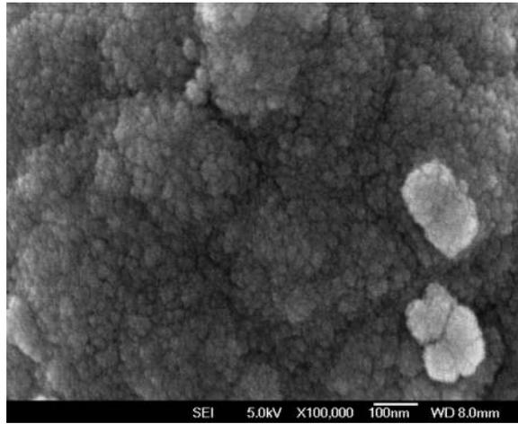
FIG. 1. The SEM image of as-deposited  $\text{Ag}_2\text{S}$  thin film prepared by chemical conversion method.
