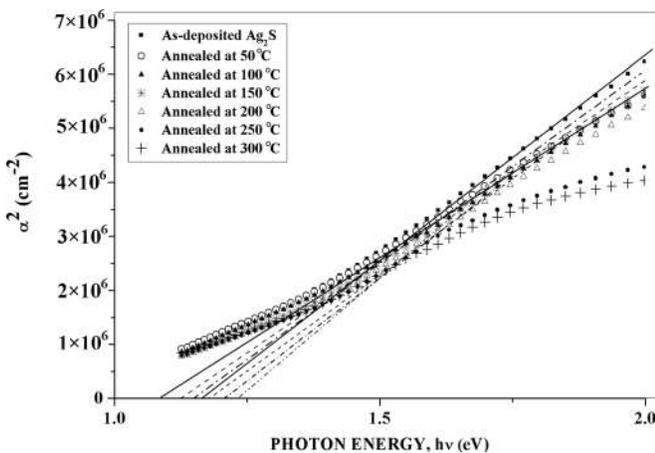
FIG. 6. The plot of  $\alpha^2$  as a function of photon energy,  $h\nu$  for the as-deposited and annealed  $Ag_2S$  thin films.
