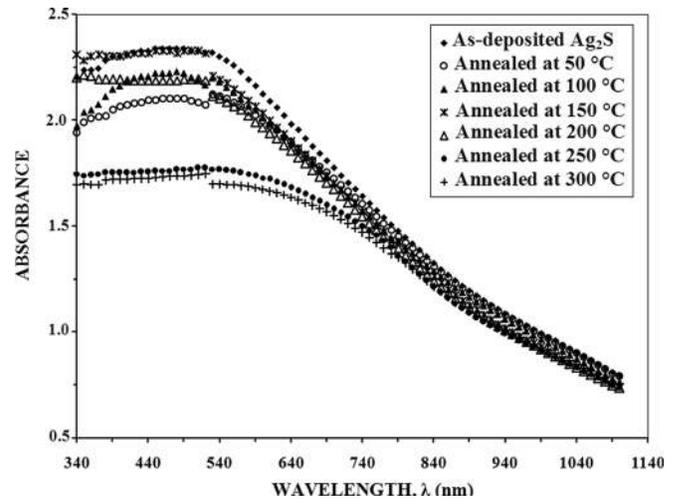
FIG. 3. Measured absorption spectra of the  $\text{Ag}_2\text{S}$  thin films, as-deposited and annealed prepared by chemical conversion method.
