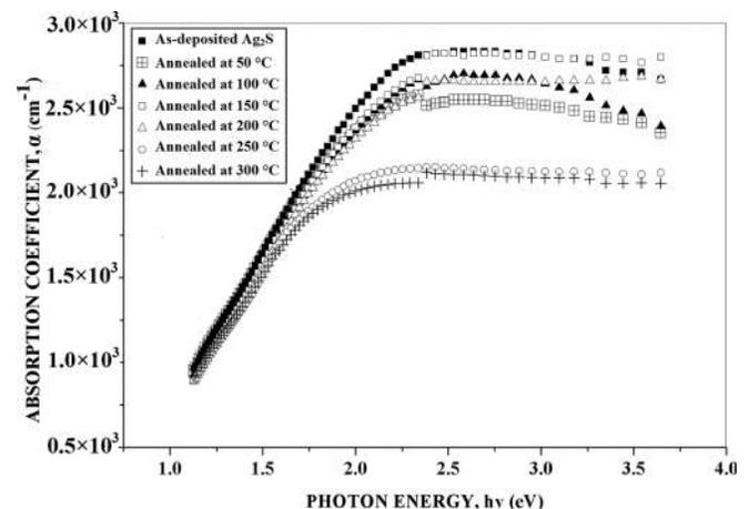
FIG. 4. Dependence of absorption coefficient,  $\alpha$ , for as-deposited and annealed  $\text{Ag}_2\text{S}$  thin films on photon energy.
