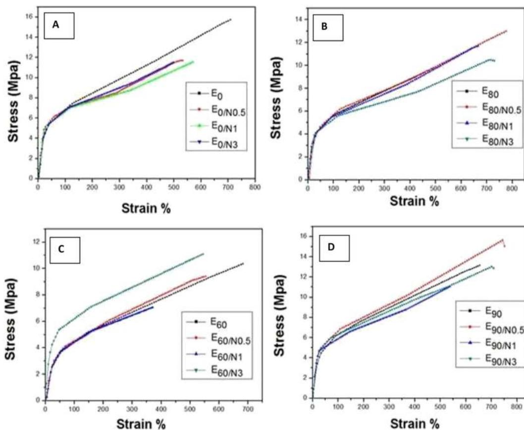
Fig. 4. Tensile stress–Strain plot of (A) POE with its different composition of clay, (B) POE/EVA (80:20) with its different composition of clay, (C) POE/EVA (60:40) with its different composition of clay, (D) POE/EVA (90:10) with its different composition of clay.
