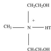
Scheme 1. Chemical structure of tallow amine used a modifier of Na-MMT.
