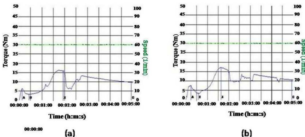
Fig. 1. Mixing torque-time profile for (a) E90 and (b) E90/N0.5.
