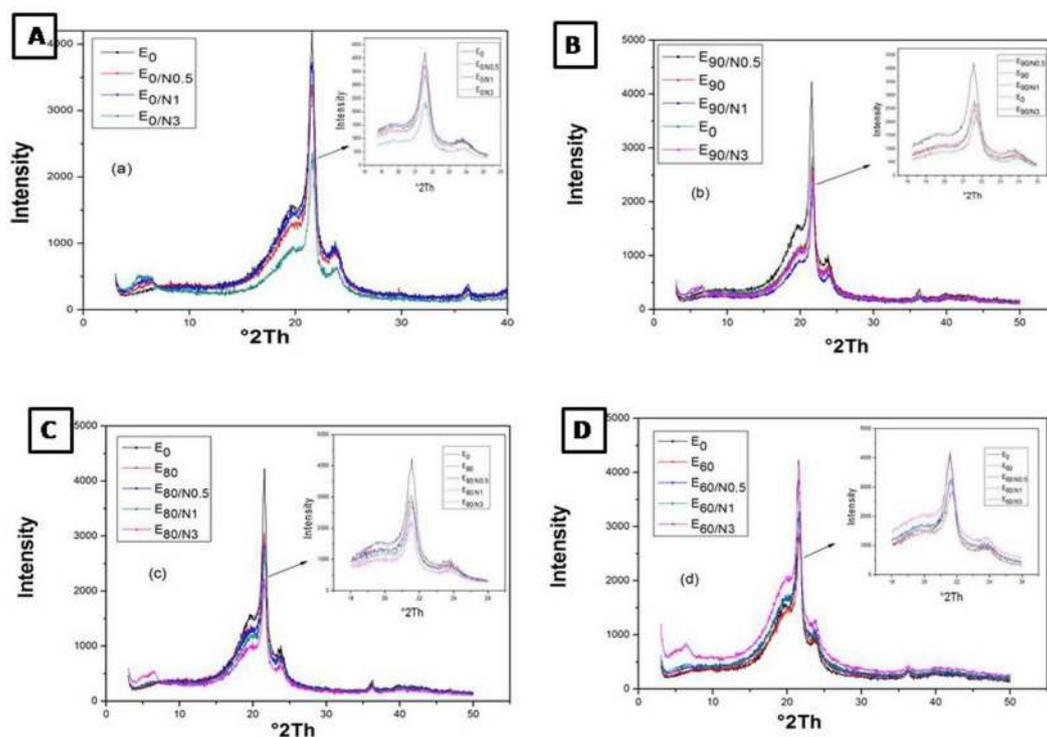
Fig. 5. XRD Spectrum of different composites of clay with (A) POE, (B) POE/EVA (90:10) blend, (C) POE/EVA (80:20) blend and (D) POE/EVA (60:40) blend.
