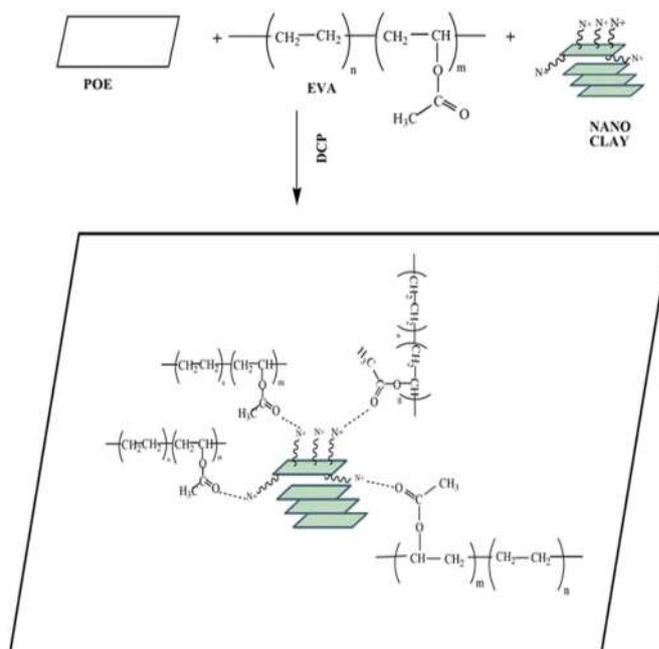
Scheme 2. Probable mechanism of interaction of nanoclay with EVA matrix.
