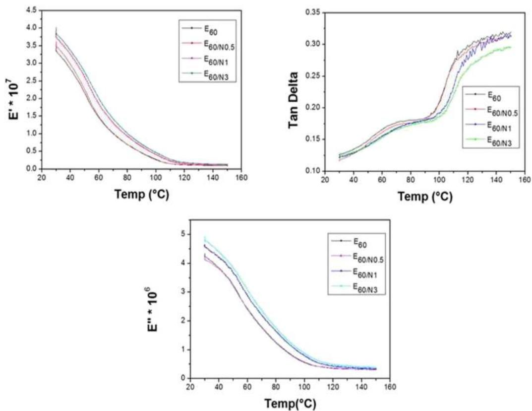
Fig. 6. DMA results of POE/EVA (60:40) blend and its different composites with clay.
