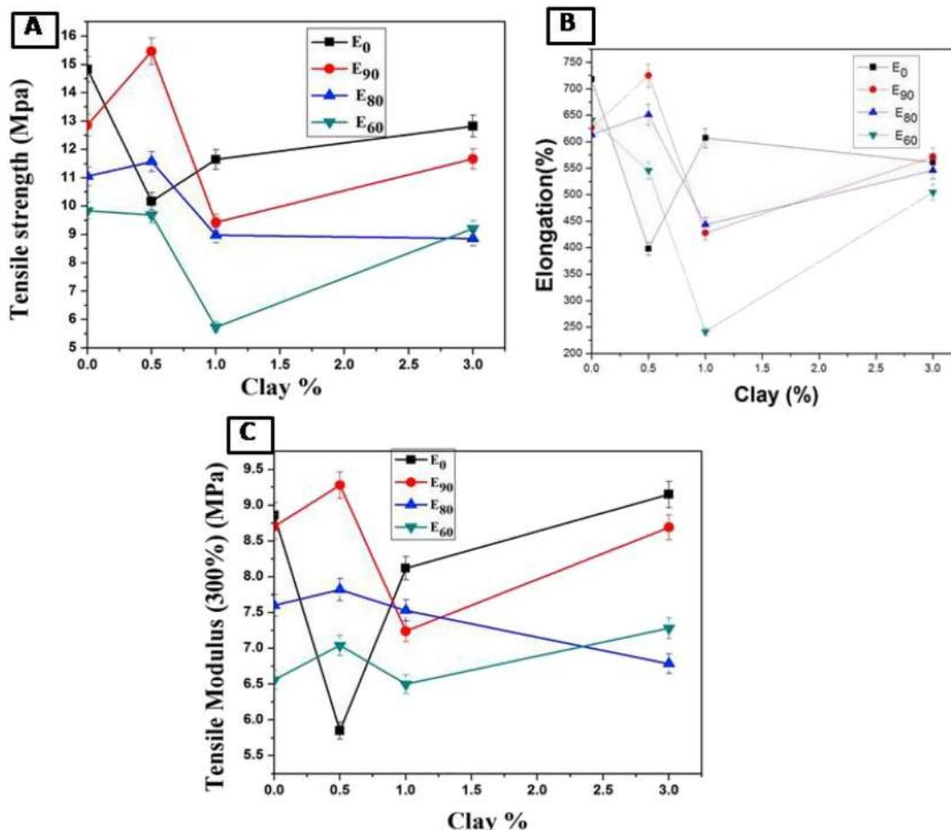
Fig. 3. Summary of mechanical properties with loading percent of clay (A) Tensile strength, (B) Elongation, (C) Tensile Modulus (300%).
