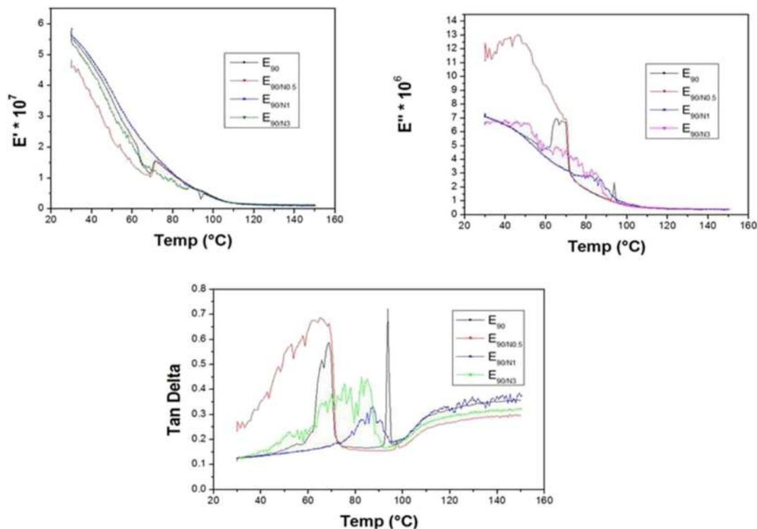
Fig. 7. DMA results of POE/EVA (90:10) blend and its different composites with clay.
