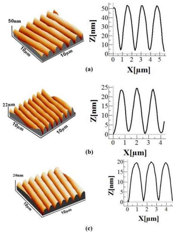
FIG. 3. AFM images along with their line scan plot of 1D grating formed with 60% Indium concentration at curing temperature of (a) 150 °C, (b) 300 °C, (c) 450 °C.
