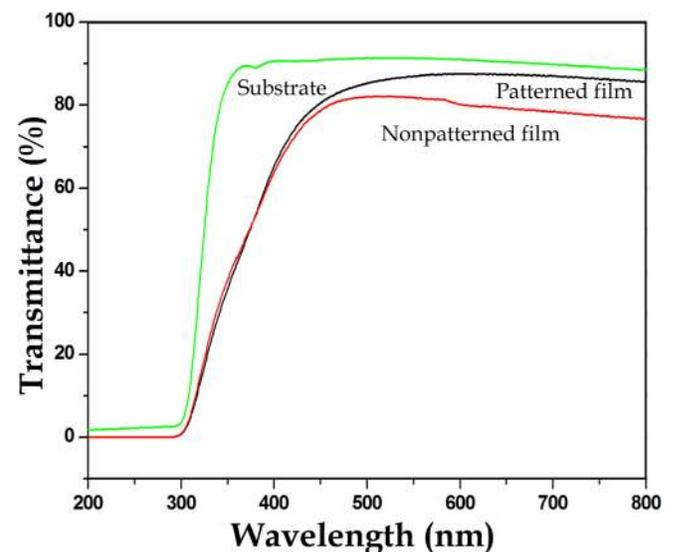
FIG. 8. UV-VIS spectrum of patterned ZI60 film along with that of unpatterned film and the glass substrate used.
