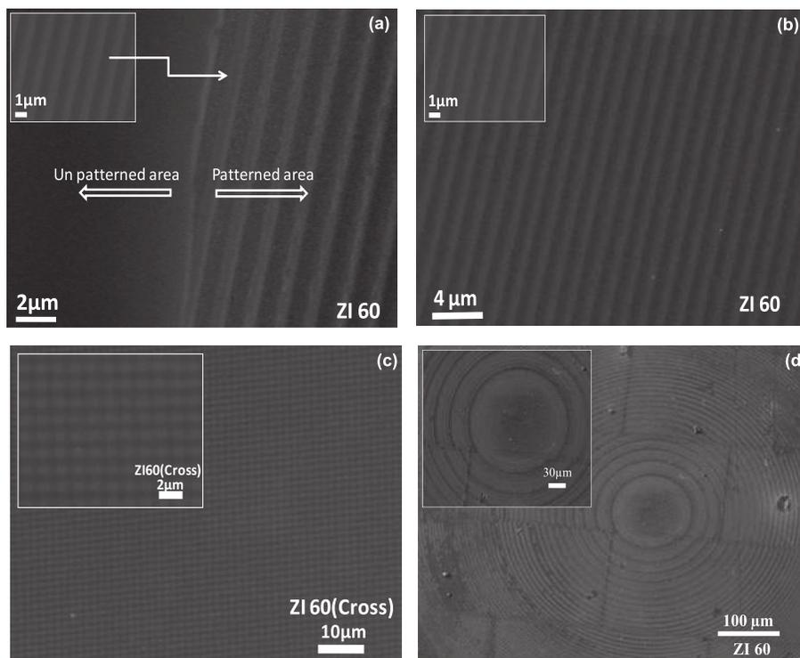
FIG. 2. FESEM images of (a) film containing patterned and non-patterned portion, (b) 1D grating pattern, (c) 2D grating pattern, (d) portion of Fresnel lens pattern. Insets show the images at higher magnification.
