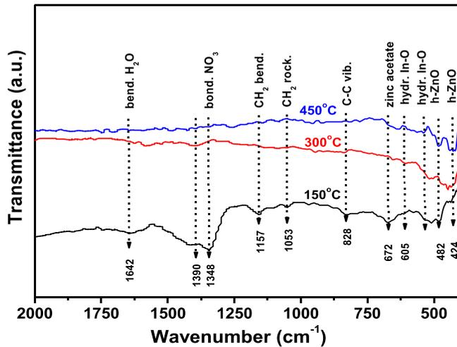
FIG. 6. Substrate corrected FTIR spectra of the ZI60 film formed after curing at three different temperatures.
