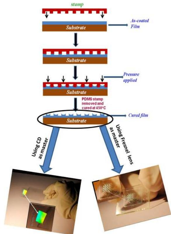
FIG. 1. Schematic of step-by-step representation of surface patterning along with pictures of formed grating patterns and Fresnel lens array.
