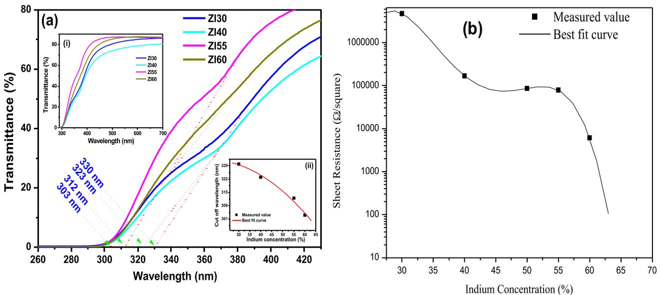
FIG. 10. (a) Determination of cut off wavelengths from UV-VIS transmission spectra of indium zinc oxide patterned films cured at 450 °C. Insets (i) and (ii) show the UV-VIS transmission spectra and the change of cut off wavelengths with indium concentration in the precursor solutions, respectively. (b) Change of sheet resistance with indium concentration in the precursor solutions.
