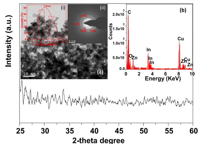
FIG. 5. XRD pattern of the grating film cured at 450 °C. Inset (a) show the TEM image of the scratched off film. Insets (i) and (ii) of inset (a) display the histogram for particle size distribution and selected area diffraction pattern of the film. Inset (b) shows the EDS data for the presence of different elements in the films network.
