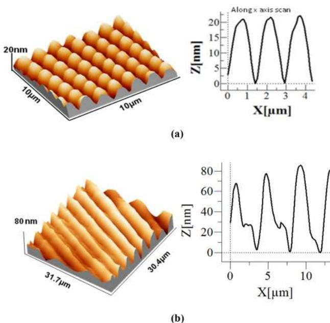
FIG. 4. AFM image along with their line scan plot of (a) 2D grating (b) portion of Fresnel lens formed with 60% indium concentration and curing temperature of 450 °C.
