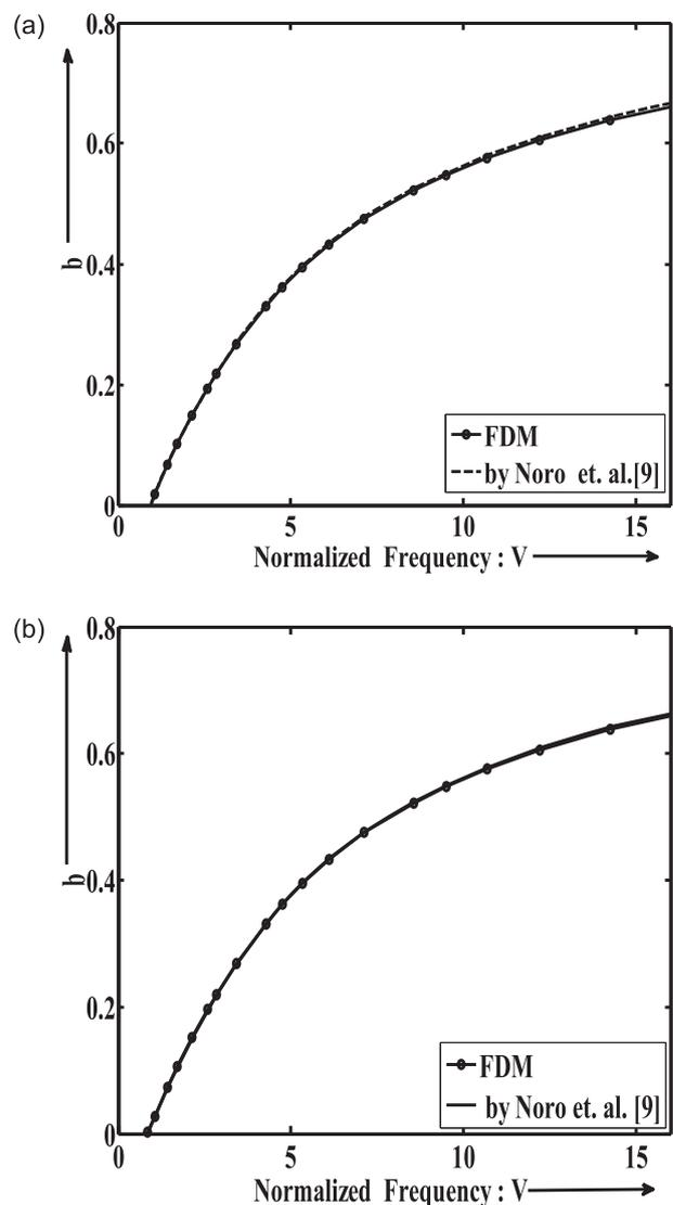
**Fig. 4:** Normalized  $b$ - $V$  plots for the exponential index profile for (a) fundamental TE mode and (b) fundamental TM mode
