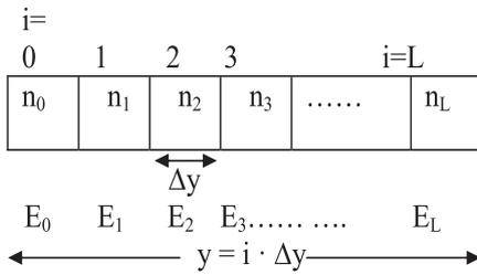
Fig. 1: Discretization of refractive index profile in transverse direction of the waveguide
