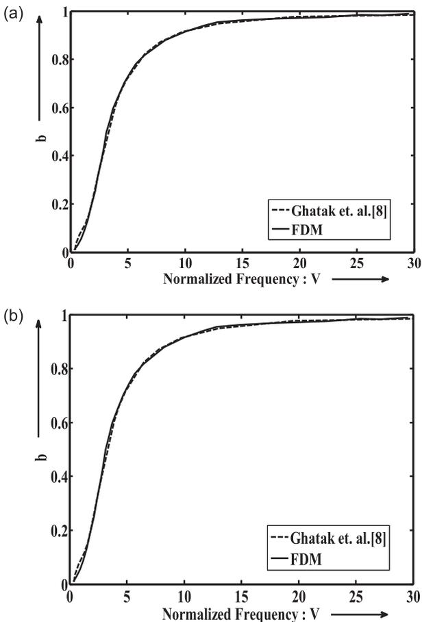
**Fig. 3:** Normalized  $b$ - $V$  plots for the step index profile for (a) fundamental TE mode and (b) fundamental TM mode
