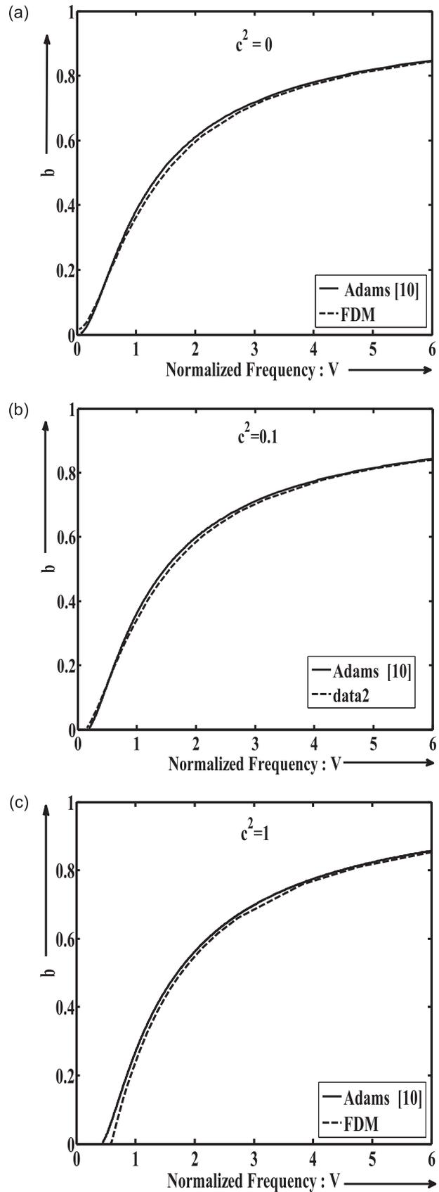
**Fig. 5:** Normalized  $b$ - $V$  plots for the general Epstein-layer profile for the asymmetric factor (a)  $c^2 = 0$ , (b)  $c^2 = 0.1$ , and (c)  $c^2 = 1$
