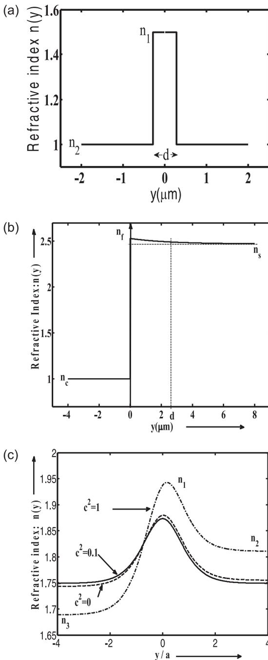
Fig. 2: Refractive index profile of (a) step index profile waveguide, (b) exponential index profile waveguide, and (c) general Epstein-layer profile for three values of the asymmetric factor  $c$  is given.
