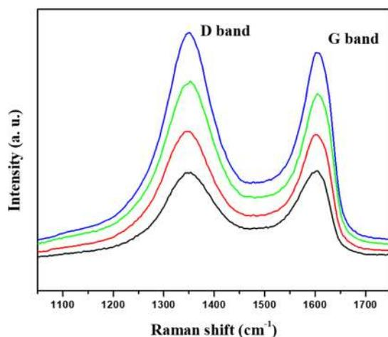
**Figure 7.** Raman spectra of GO (black), APTES@GO (red), AA@APTES@GO (green), and Cu@AA@APTES@GO (blue).
