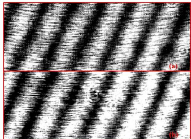
FIG. 2. A typical observed fringe pattern obtained from the MZI setup for (a) zero applied field and (b) applied field for half wave phase shift. Similar fringe pattern can be obtained for different types of LiNbO<sub>3</sub> crystals.
