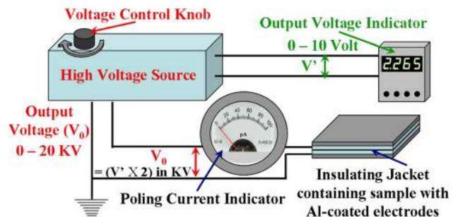
FIG. 4. High voltage electric field poling setup.
