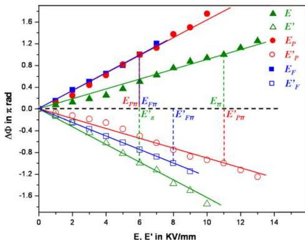
FIG. 3. Phase variation with the applied field for as-bought LiNbO<sub>3</sub> crystal (green line), stable domain inverted LiNbO<sub>3</sub> crystal (red line), and frustrated domain inverted LiNbO<sub>3</sub> crystal (blue line).
