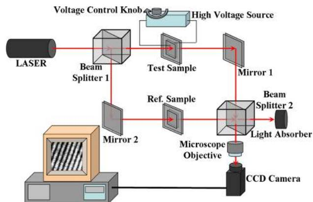
FIG. 1. Setup for the measurement of internal field in  $\text{LiNbO}_3$  crystals.
