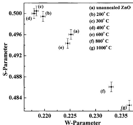
FIG. 7. Variation of  $S$  parameter with  $W$  parameter for unannealed and annealed ZnO samples.
