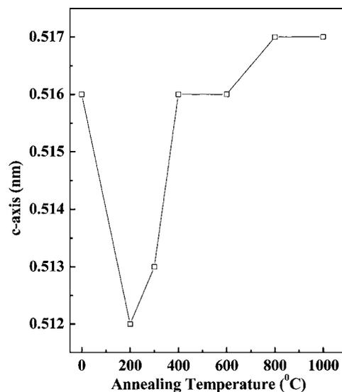
FIG. 6. Variation of  $c$ -axis lattice parameter of ZnO with annealing temperature.
