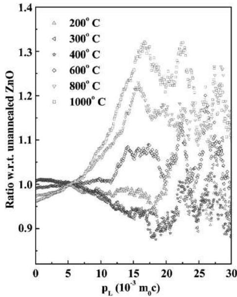
FIG. 4. Ratio curve of the experimental electron-positron momentum distributions for the annealed ZnO samples with respect to the same unannealed ZnO.
