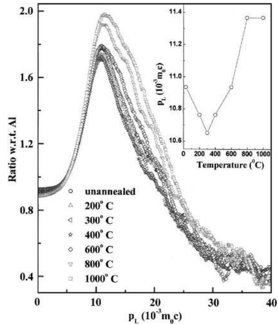
FIG. 3. Ratio curves of the experimental electron-positron momentum distributions for unannealed and annealed ZnO samples with respect to standard electron-positron momentum distribution of a defect-free Al single crystal. The inset shows the relative position of the ratio curve peaks for the ZnO samples with annealing temperature.
