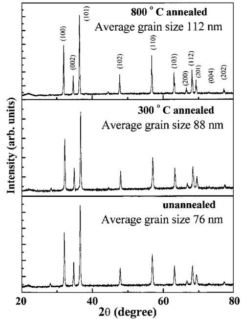
FIG. 1. X-ray-diffraction patterns for the unannealed and annealed ZnO samples.
