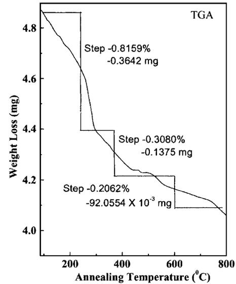
FIG. 5. TGA curve of the unannealed ZnO sample.
