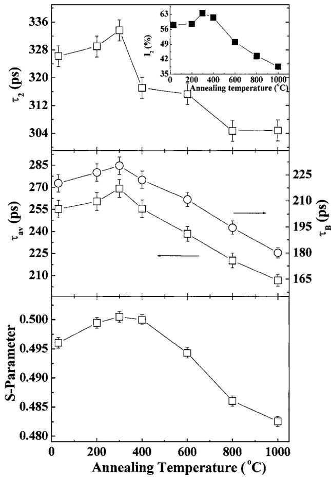
FIG. 2. Variation of  $\tau_2$  (positron lifetime at defects), average position lifetime ( $\tau_{av}$ ), bulk positron lifetime ( $\tau_B$ ), and  $S$  parameter with annealing temperature for the ZnO samples. The inset shows the variation of  $I_2$  (intensity corresponding to  $\tau_2$ ) with annealing temperature. The annealing temperature of the unannealed ZnO sample has been taken as 30 °C (room temperature).
