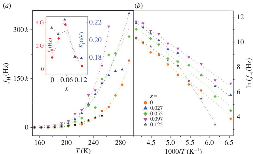
**Figure 5.** Temperature dependence of (a) hopping frequency,  $f_H$  versus  $T$  and (b)  $\log(f_H)$  versus  $1000/T$  for  $Cu_{1-x}Fe_xO$  ( $0 \leq x \leq 0.125$ ). The dotted lines represent fitted spectra.
