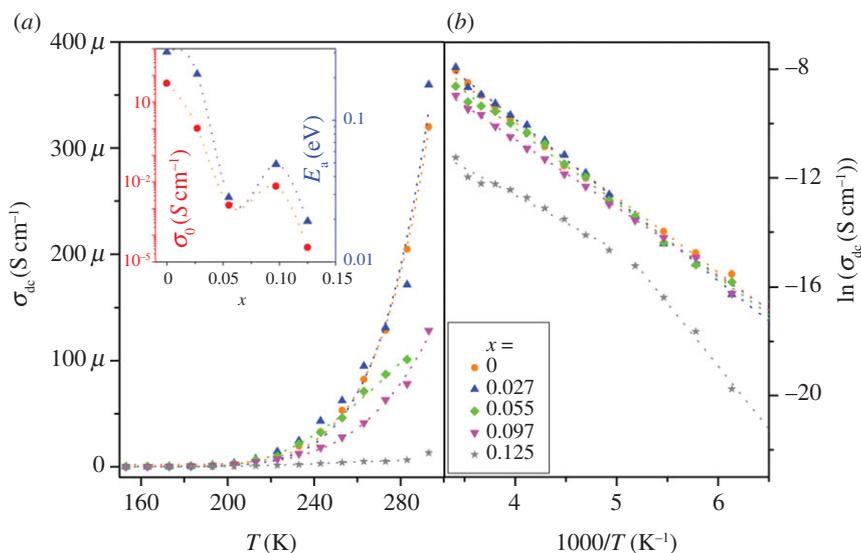
**Figure 4.** Temperature dependence of (a) DC conductivity,  $\sigma_{dc}$  versus  $T$  and (b)  $\log(\sigma_{dc})$  versus  $1000/T$  for  $\text{Cu}_{1-x}\text{Fe}_x\text{O}$  ( $0 \leq x \leq 0.125$ ). The dotted lines represent fitted spectra.
