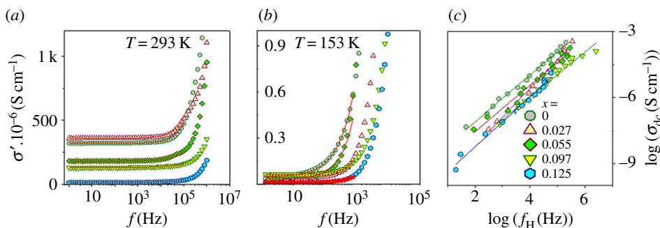
**Figure 3.** Frequency spectra of the real conductivity ( $\sigma'$ ) at (a) 293 K, (b) 153 K and (c) Barton–Nakajima–Namikawa (BNN) plots for  $\text{Cu}_{1-x}\text{Fe}_x\text{O}$  ( $0 \leq x \leq 0.125$ ). The solid lines are obtained from the Jonscher Law fit of complex conductivities.
