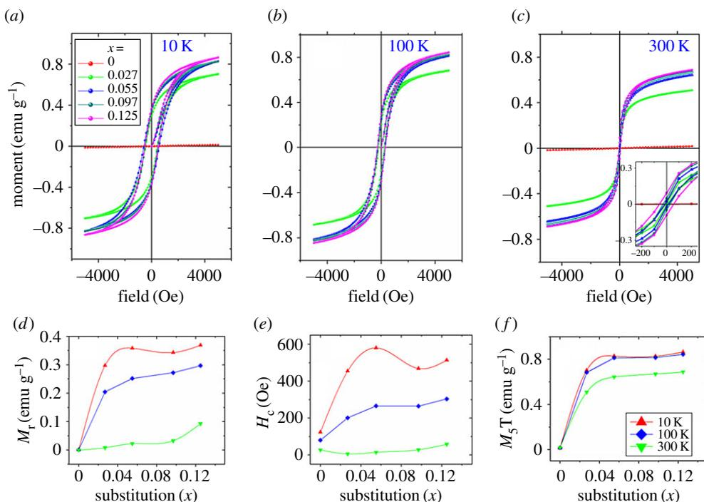
**Figure 6.** Ferromagnetic hysteresis loops ( $M$ – $H$ ) at (a) 10 K, (b) 100 K, (c) 300 K, (d) remnant magnetization ( $M_r$ ), (e) coercivity ( $H_c$ ) and (f) magnetization ( $M_{5T}$ ) versus substitution at 5 T field for  $\text{Cu}_{1-x}\text{Fe}_x\text{O}$  ( $0 \leq x \leq 0.125$ ) samples.
