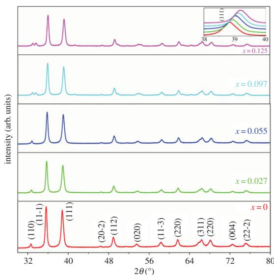
**Figure 1.** XRD pattern of  $\text{Cu}_{1-x}\text{Fe}_x\text{O}$  ( $0 < x < 0.125$ ) samples revealing a systematic shift in (111) peak towards larger angles.
