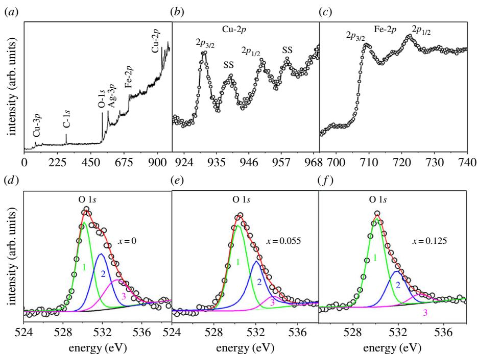
**Figure 2.** (a) XPS survey spectrum and high-resolution scans of (b) Cu 2p and (c) Fe 2p of  $\text{Cu}_{0.875}\text{Fe}_{0.125}\text{O}$ . The O 1s edge spectra of  $\text{Cu}_{1-x}\text{Fe}_x\text{O}$  samples; (d)  $x = 0$ , (e)  $x = 0.055$  and (f)  $x = 0.125$ .
