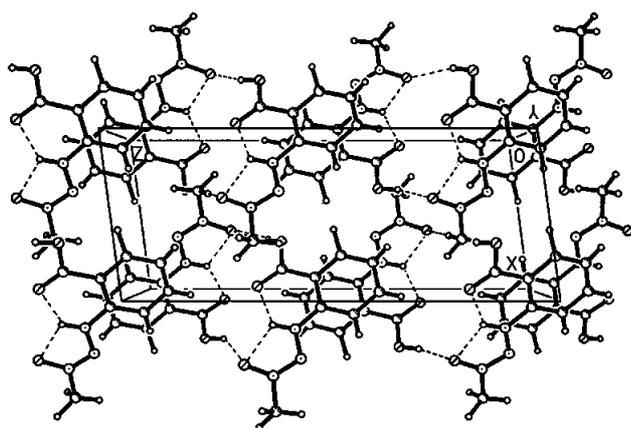
Fig. 3 A unit cell drawing of the packing arrangement and dashed lines indicate N-H...O and O-H...O hydrogen bonds..
