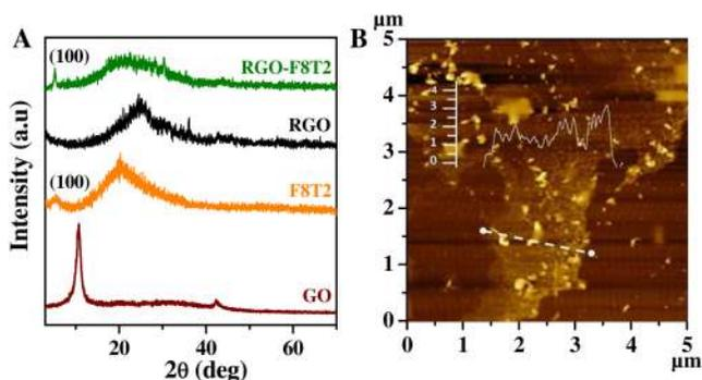
**FIG. 1.** (a) XRD patterns of the GO, F8T2, RGO, and RGO-F8T2 composites. (b) AFM image of RGO-F8T2 composite films on a silicon wafer.
