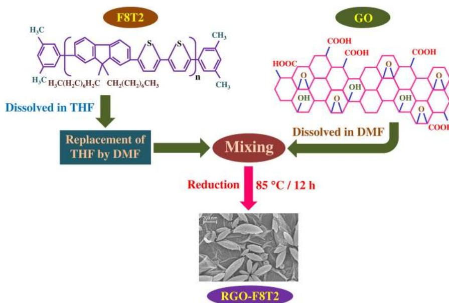
**SCHEME 1.** Schematic representation of the synthesis of the RGO-F8T2 composite.
