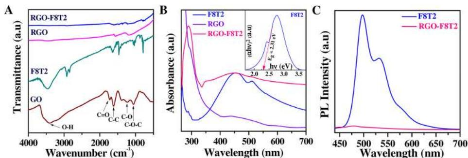
**FIG. 2.** (a) FTIR spectra of the GO, F8T2, RGO, and RGO-F8T2 composites. (b) Optical absorption spectra of the F8T2, RGO, and RGO-F8T2 composites. Plot of  $(\alpha h\nu)^2$  vs photon energy of F8T2 is shown in the inset. (c) Photoluminescence spectra of the F8T2 and the RGO-F8T2 composites.
