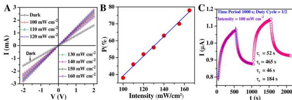
**FIG. 6.** I–V characteristics for a RGO–F8T2 composite thin film device under the dark condition and under different illumination intensities. (b) The variation of photosensitivity with illuminated intensity. (c) Current versus time for two consecutive cycles as the light was turned on and off.
