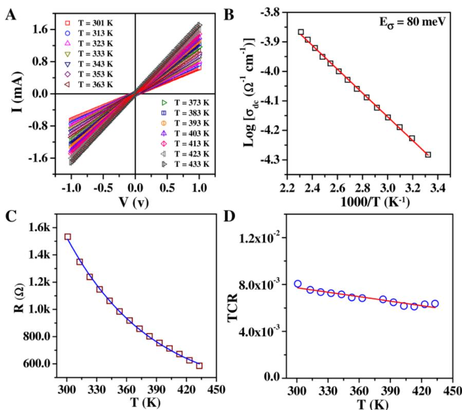
**FIG. 3.** (a) I-V characteristics of the RGO-F8T2 composite pellet. (b) The Arrhenius behaviour of dc conductivity with its straight line fit. Variation of (c) resistance and (d) TCR with temperature of the RGO-F8T2 composite.
