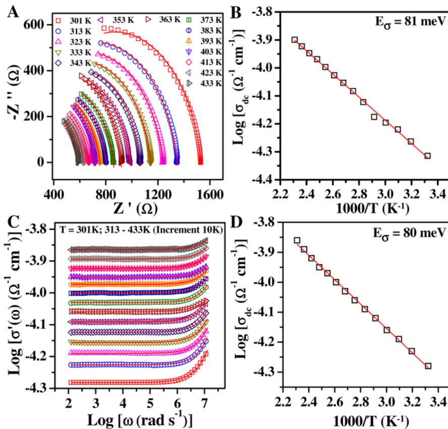
FIG. 4. (a)  $Z'$  vs  $Z''$  curve with equation of circle fits of the RGO-F8T2 composite pellet. (b) The Arrhenius behaviour of dc conductivity with its straight line fit. (c) The frequency spectra of the real conductivity  $\sigma'(\omega)$  for different temperatures. The solid lines are the best fits to Eq. (5). (d) The Arrhenius behaviour of dc conductivity with its straight line fit.
