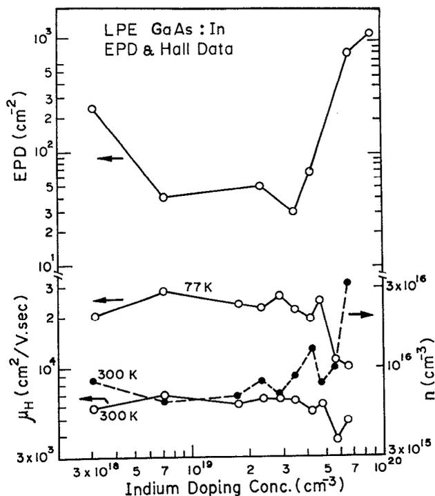
FIG. 1. Etch pit density (EPD), Hall mobility ( $\mu_H$ ) and Hall carrier concentrations ( $n$ ) of GaAs layers grown with different amounts of indium doping.
