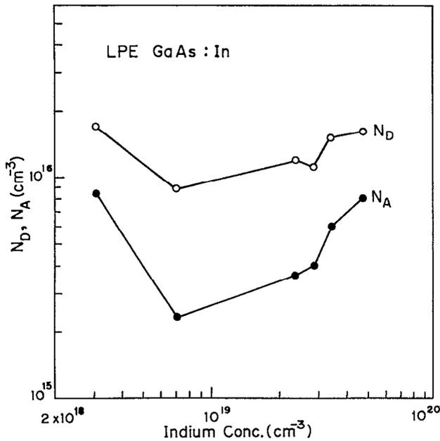
FIG. 2. Donor concentrations ( $N_D$ ) and acceptor concentrations ( $N_A$ ) calculated from the analysis of the Hall measurement data of GaAs doped with indium.
