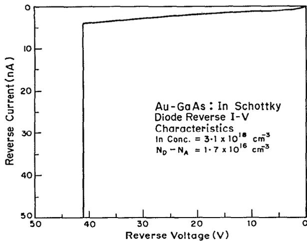
FIG. 4. Reverse current-voltage ( $I$ - $V$ ) characteristics of a typical Au-GaAs:In Schottky barrier diode.
