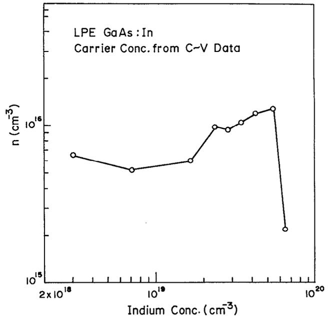
FIG. 3. 300 K free carrier concentrations ( $n$ ) obtained from the *C-V* measurements of gold Schottky barrier diodes fabricated on In-doped GaAs layers.
