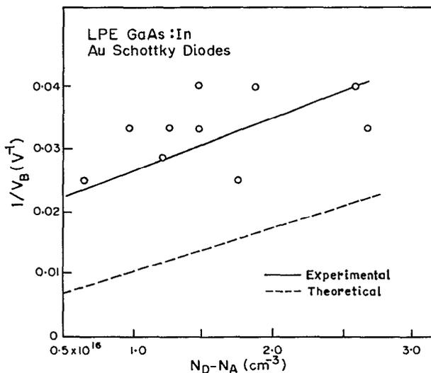
FIG. 5. Inverse of breakdown voltage  $V_B$  of Au-GaAs:In diodes plotted as a function of the measured values of  $N_D - N_A$ . The solid line is the best fit to the experimental data whereas the dashed line represents values calculated from theoretical models.
