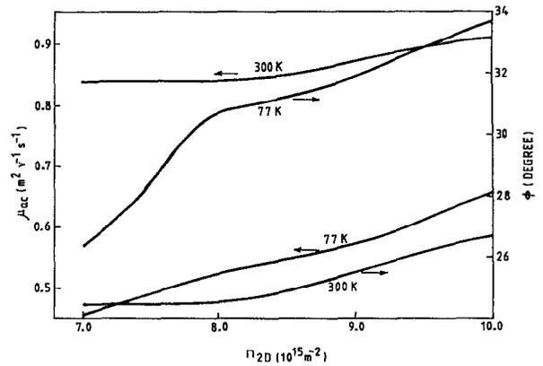
FIG. 4. Plot of  $\mu_{ac}$  and  $\phi$  with  $n_{2D}$  at 200 GHz for 77 and 300 K. The other parameters have the same values as in Fig. 1.
