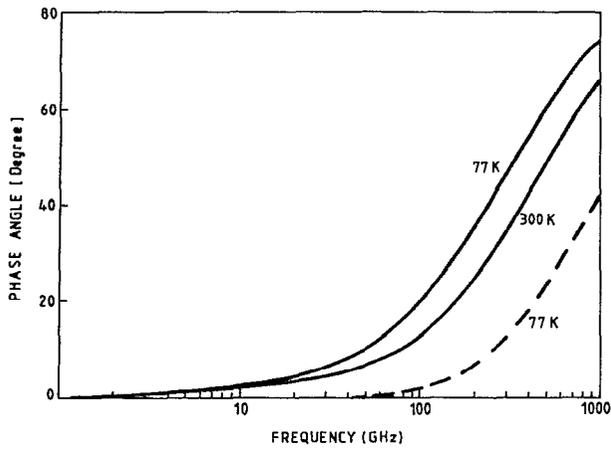
FIG. 2. Plot of the phase lag  $\phi$  of the drift velocity behind the applied signal versus frequency for 77 and 300 K. The parameter values are the same and the solid and the dashed curves have the same significance as in Fig. 1.
