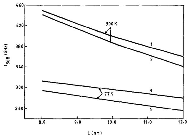
FIG. 5. Plot of the 3 dB cut-off frequency  $f_{3dB}$  vs the channel width  $L$  for 77 and 300 K. (1), (4):  $n_{2D} = 10^{16} \text{ m}^{-2}$ ; (2), (3):  $n_{2D} = 8 \times 10^{15} \text{ m}^{-2}$ . The other parameters are identical to those of Fig. 1.
