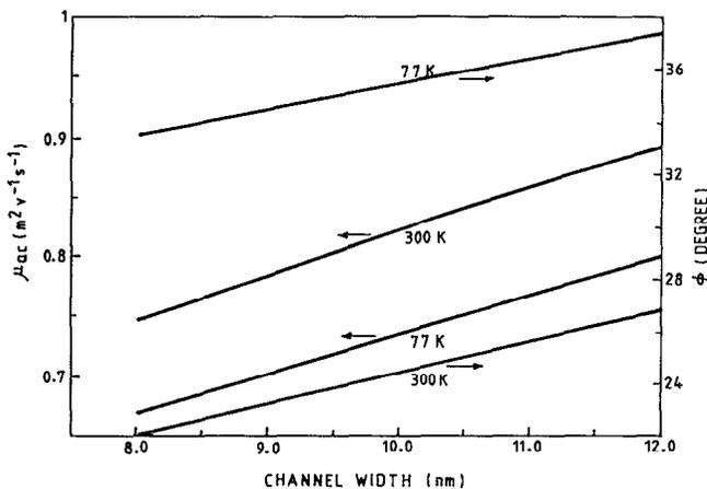
FIG. 3. Variation of  $\mu_{ac}$  and  $\phi$  with  $L$  at a frequency of 200 GHz for 77 and 300 K. The other parameters are the same as in Fig. 1.
