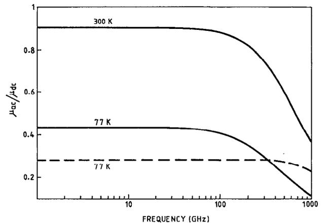
FIG. 1. Variation of  $\mu_{ac}/\mu_{dc}$  with frequency for 77 and 300 K. Solid curves are for  $L = 10$  nm,  $n_{2D} = 10^{16}$  m<sup>-2</sup>, and  $N_i = 10^{21}$  m<sup>-3</sup>. The dashed curve is for a nondegenerate system with  $L = 10$  nm (Ref. 16).
