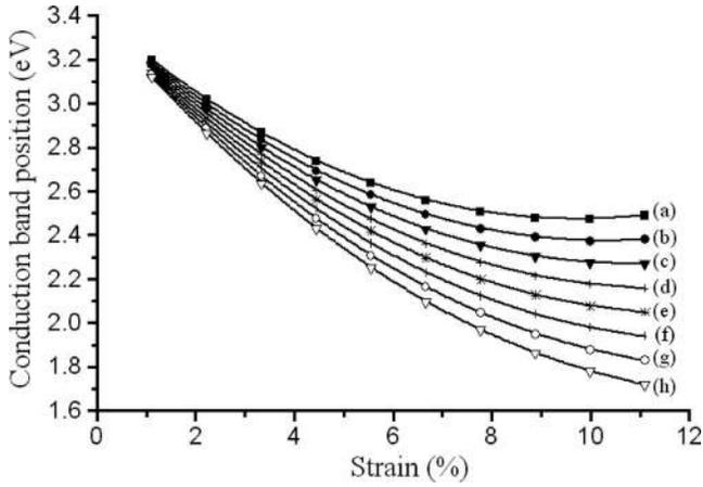
FIG. 2. Variations of conduction band positions with strain. Band gap of InN ( $E_{g,\text{InN}}$ ) is varied as (a) 2.1 eV, (b) 1.9 eV, (c) 1.7 eV, (d) 1.5 eV, (e) 1.3 eV, (f) 1.1 eV, (g) 0.9 eV, and (h) 0.7 eV.
