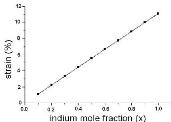
FIG. 1. Variation of strain with indium mole fraction in an  $\text{In}_x\text{Ga}_{1-x}\text{N}/\text{GaN}$  system.
