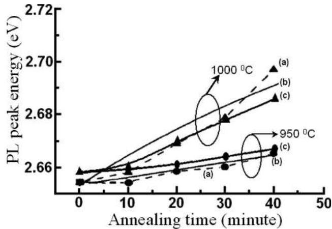
FIG. 5. Variation of PL peak energy with annealing time (a) found experimentally, (b) calculated by Chuo *et al.*, and (c) calculated using Eqs. (4) and (5).
