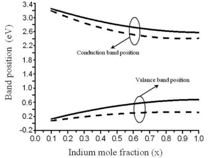
FIG. 4. Band positions of  $\text{In}_x\text{Ga}_{1-x}\text{N}/\text{GaN}$  system. The continuous curves show the variation without considering strain and the dashed curves show the variation considering strain.
