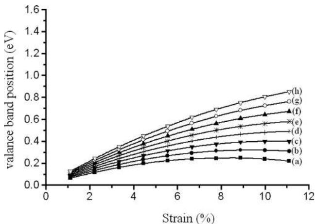
FIG. 3. Dependence of valence band positions on strain. Band gap of InN ( $E_{g,\text{InN}}$ ) is varied as (a) 2.1 eV, (b) 1.9 eV, (c) 1.7 eV, (d) 1.5 eV, (e) 1.3 eV, (f) 1.1 eV, (g) 0.9 eV, and (h) 0.7 eV.
