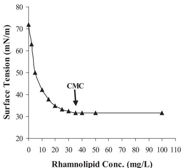
Fig. 2 Surface tension (mN/m) versus rhamnolipid concentration (mg/L)
