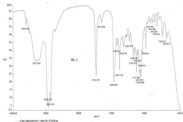
Fig. 1 FTIR spectrum of extracted rhamnolipid
