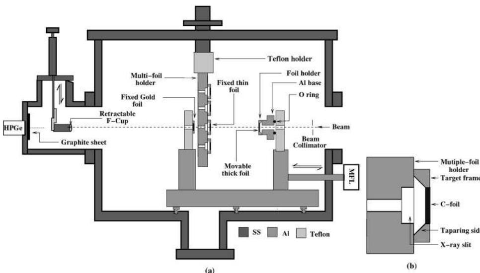
FIG. 2. (a) Cross-sectional view of the experimental chamber (not to scale); (b) enlarged view of a fixed thin foil frame in the multiple-foil holder.
