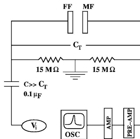
FIG. 3. Arrangement for the measurement of the minimum distance between the two foils. FF indicates the fixed foil, MF the movable foil,  $C_T$  the capacitance due to the two foils, and  $C$  the capacitance of the dc filtering capacitor.
