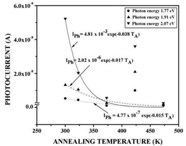
FIG. 2. The variation of photocurrent of the ZnSe thin film with annealing temperature for different sub-band gap photon energies.
