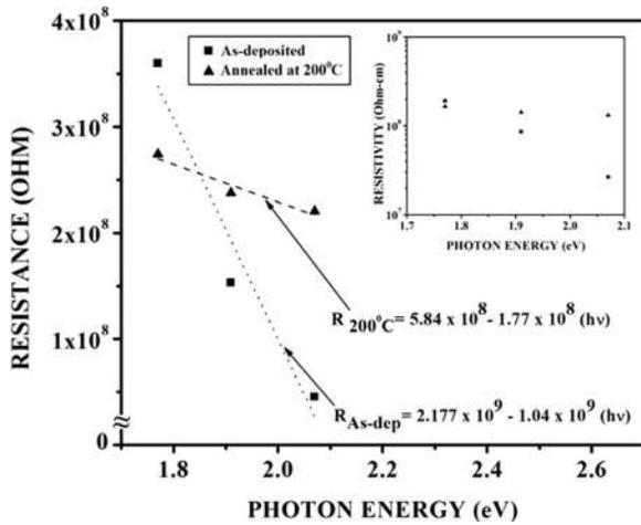
FIG. 4. The variation of resistance of ZnSe thin film with the photon energy for the as-deposited sample and the sample annealed at 200°C. The inset shows the variation of the resistivity of the material with the photon energy.
