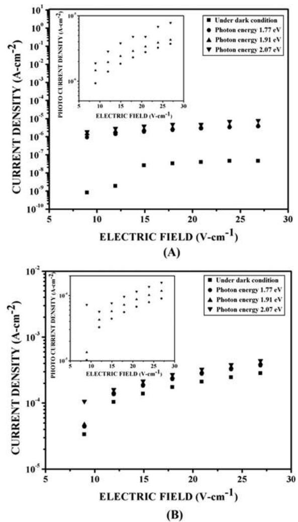
FIG. 8. The current density vs. electric field characteristics of as-deposited (a) and 200 °C annealed (b) CdS thin films under sub-band gap optical illumination. The insets in (a) and (b) show the variations of the photocurrent density with electric field for as-deposited and annealed CdS samples under sub-band gap optical illumination.
