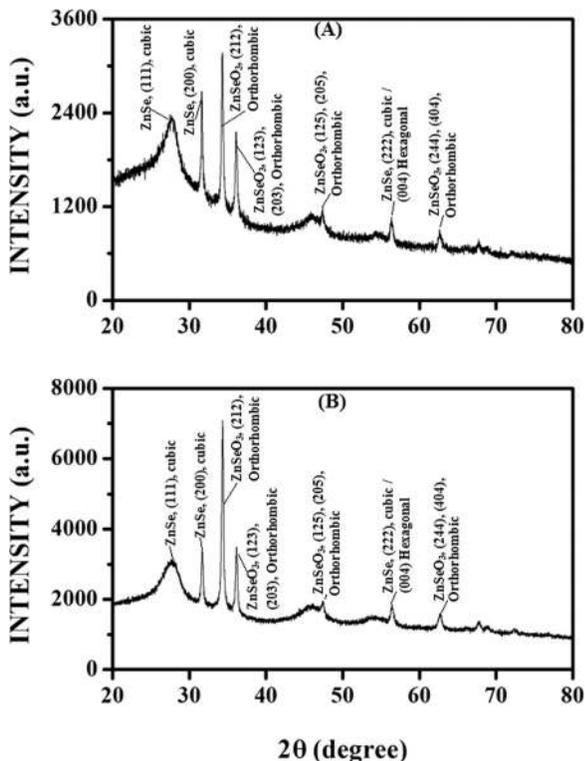
FIG. 7. The XRD pattern of the ZnSe thin film deposited by the chemical bath deposition technique. (a) As-deposited sample and (b) sample annealed at 200 °C.
