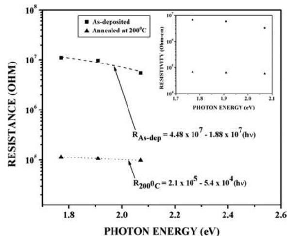
FIG. 9. The variation of resistance of the CdS thin film with the photon energy for the as-deposited sample and the sample annealed at 200 °C. The inset shows the variation of the resistivity of the material with the photon energy.
