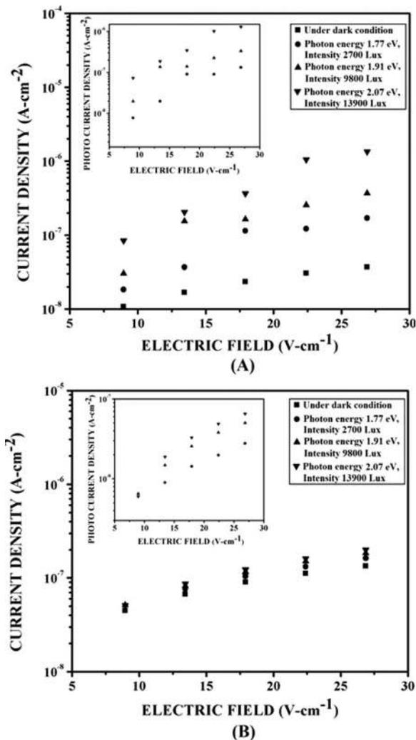
FIG. 1. The current density vs. electric field characteristics of as-deposited (a) and 2000 °C annealed (b) ZnSe thin films under sub-band gap optical illumination. The insets in (a) and (b) show the variations of the photocurrent density with electric field for as-deposited and annealed ZnSe samples under sub-band gap optical illumination.
