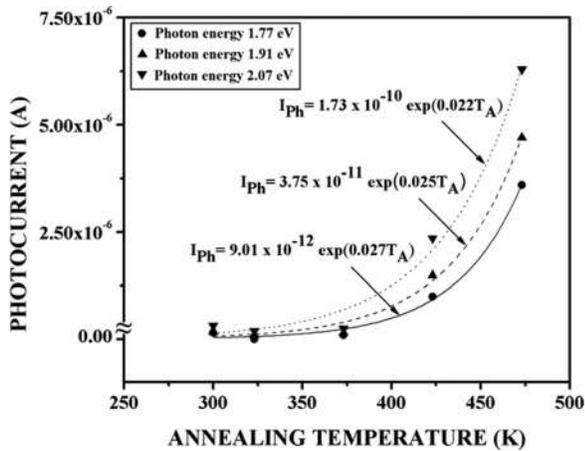
FIG. 10. The variation of the photocurrent of the CdS thin film with annealing temperature for different sub-band gap optical energies.
