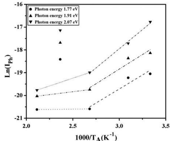
FIG. 3. The logarithmic variation of the photocurrent of ZnSe thin film with the inverse annealing temperature.
