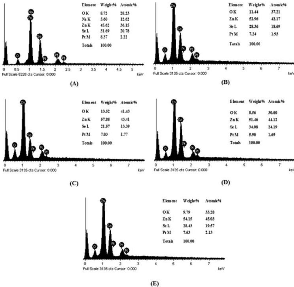
FIG. 6. The EDS graphs for the as-deposited and annealed ZnSe samples. (a) As-deposited, (b) annealed at 50 °C, (c) annealed at 100 °C, (d) annealed at 150 °C, and (e) annealed at 200 °C.
