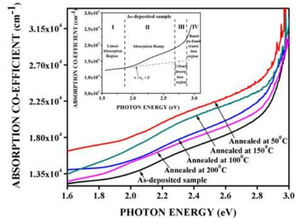
FIG. 5. The variation of the optical absorption co-efficient of the as-deposited and annealed ZnSe thin films. The inset shows the four different optical absorption regions for the as-deposited sample.
