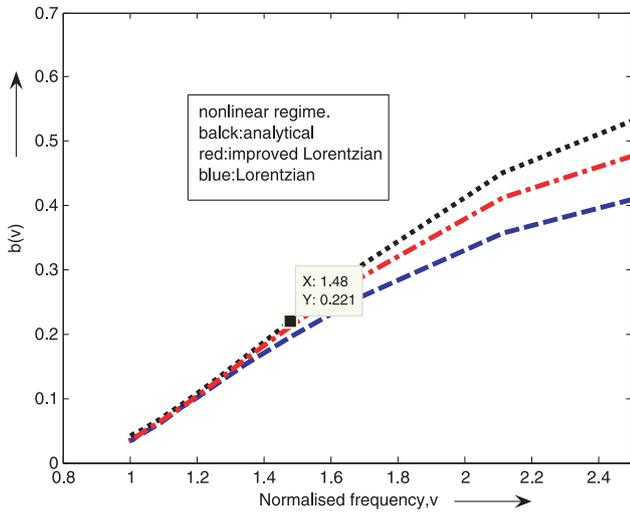
Fig. 6:  $b(V)$  (normalised propagation constant) vs.  $V$  (normalised frequency)
