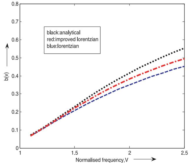
**Fig. 5:**  $b(V)$  (normalized propagation constant) vs.  $V$  (normalised frequency)
