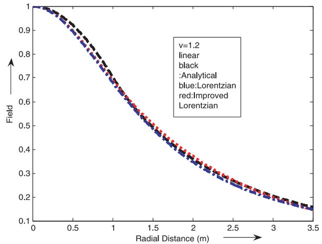
Fig. 1: Field vs. radial distance along the optical fiber at  $V = 1.2$
