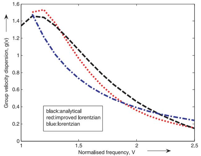
Fig. 9:  $g(V)$  (normalized wave guide dispersion) vs.  $V$  (normalised frequency)
