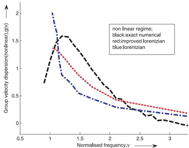
Fig. 10:  $g(V)$  (normalized wave guide dispersion) vs.  $V$  (normalised frequency)
