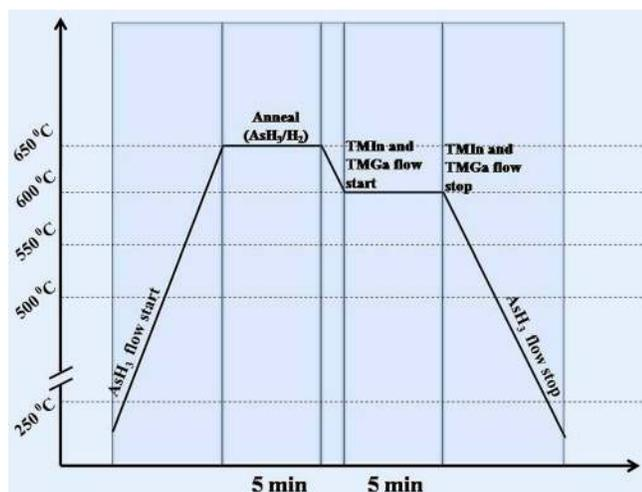
FIG. 1. Temperature-time profile of the growth process.
