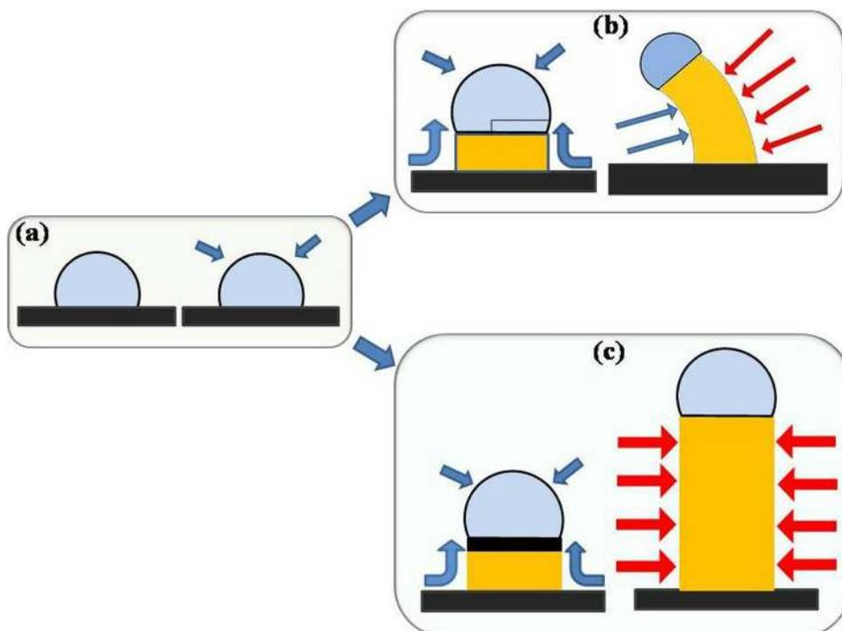
FIG. 4. Schematic of NW growth. The radius of monolayer affecting the morphology of NW. (a) The catalyst forms a droplet when heated to eutectic temperature. Supersaturation occurs after adsorbing the precursors, and nucleation occurs at TPP. (b) The nucleus covers a fraction of interface area between the catalyst and the substrate. (c) The nucleus covers the entire interface area.
