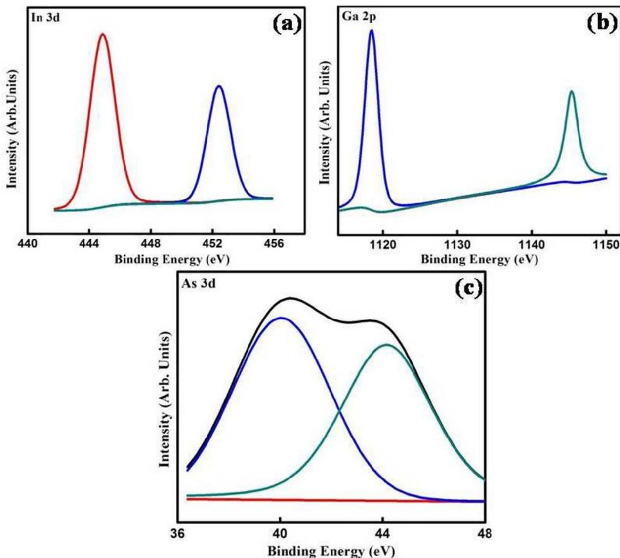
FIG. 7. XPS signals of (a) In 3d, (b) Ga 2p, and (c) As 3d.
