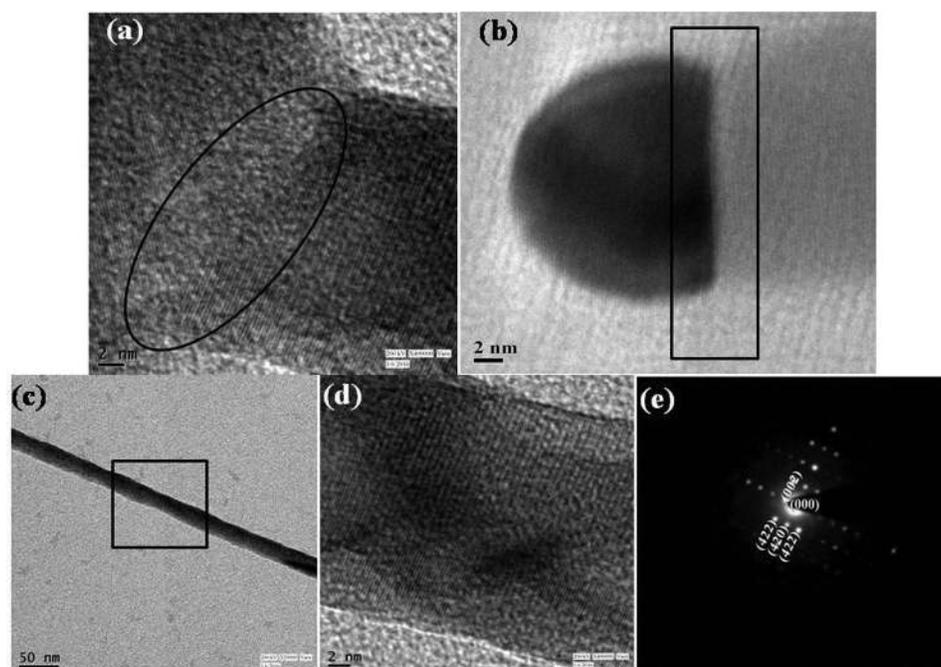
FIG. 6. (a) HRTEM image of the interface between the nanoparticle and NW for S2. It shows the case for which the nucleus covers a fraction of area on the nanoparticle-nanowire interface. (b) HRTEM image of the interface between the nanoparticle and NW for S3. It shows the case when the nucleus covers the entire interface area. (d) BF HRTEM images of S3 NW show single crystalline structure. (e) The indexed SAED pattern of S3 shows defect free zinc blend structure.
