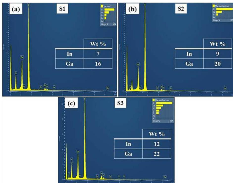
FIG. 5. EDX spectrum of (a) S1, (b) S2, and (c) S3.
