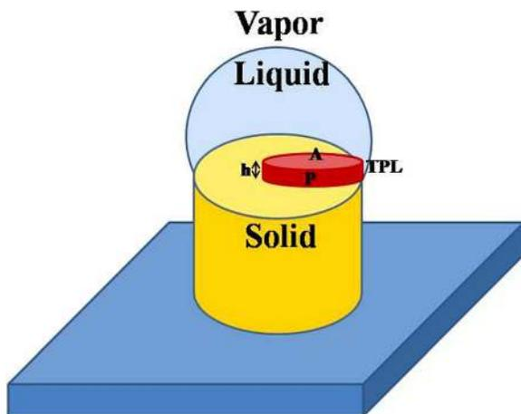
FIG. 3. Nucleation of monolayer island at triple phase boundary. The red disk is shown as the nucleus. A certain fraction of the total substrate-catalyst interface is covered at a specific level of supersaturation.
