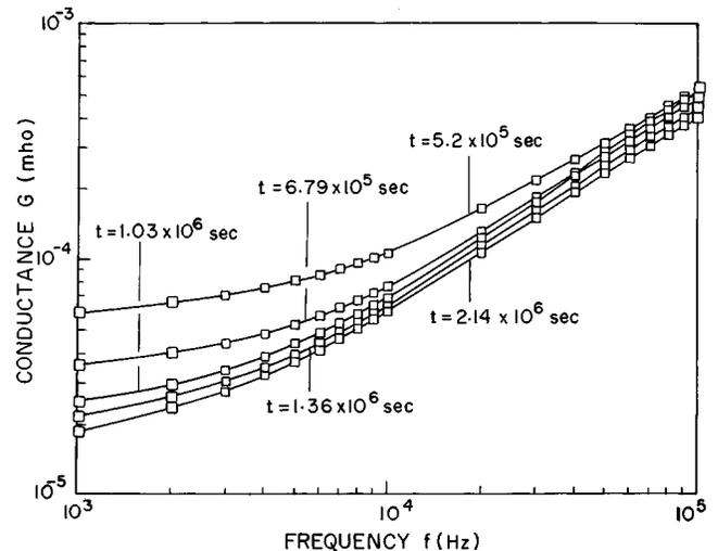
FIG. 5. Conductance-frequency plots of a Ni-*p*-Si contact at different aging times.
