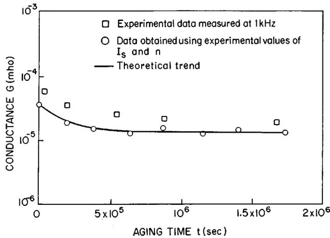
FIG. 9. Variation of low frequency conductance of a Ni-p-Si contact with the aging time.
