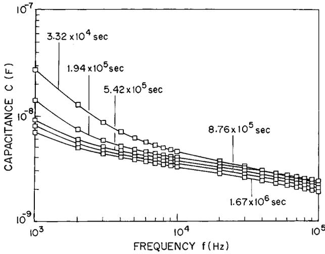
FIG. 6. Capacitance–frequency plots of a Ni–p-Si contact at different aging times.
