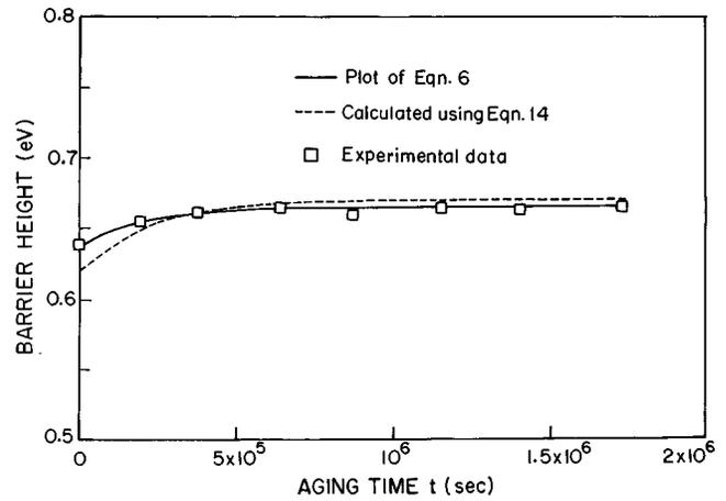
FIG. 4. Variation of the barrier height of a Ni-*p*-Si contact as a function of the aging time.
