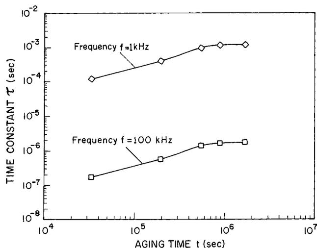
FIG. 11. Plot of low and high frequency time constants of interface states as a function of the aging time. The results were obtained using Eqs. (12) and (13).
