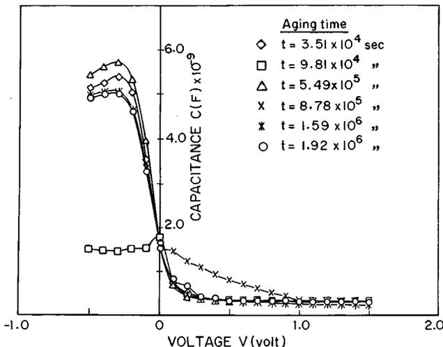
FIG. 7. Capacitance–voltage characteristics of a Ni–p-Si contact at different aging times.
