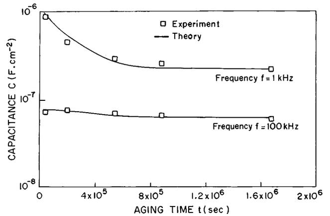
FIG. 10. Variation of low and high frequency capacitance of a Ni-p-Si contact as a function of the aging time. The continuous curves represent theoretical plots generated with the help of Eqs. (8)–(14). The interface state densities at frequencies of 1 and 100 kHz are considered to be  $7 \times 10^{12}$  and  $3.9 \times 10^{11} \text{ cm}^{-2} \text{ eV}^{-1}$ , respectively.
