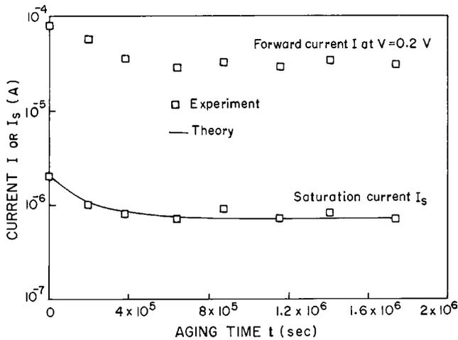
FIG. 2. Variation of current as a function of the aging time in a Ni-*p*-Si contact.
