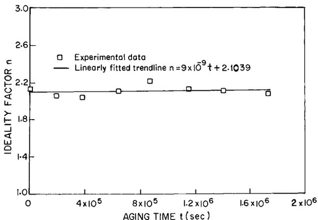
FIG. 3. Variation of the ideality factor of a Ni-*p*-Si contact with the aging time.
