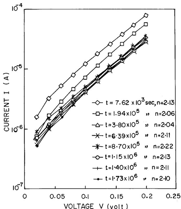
FIG. 1. Current–voltage characteristics of a Ni–*p*-Si contact at different aging times.
