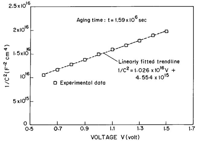
FIG. 8.  $1/C^2$  vs  $V$  characteristics of a Ni–p-Si contact at aging time  $t = 1.59 \times 10^6$  s.
