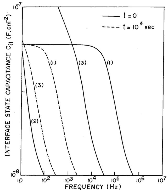
FIG. 11. The variation of interface state capacitance of a MIS tunnel device as a function of bias voltage and interface reaction. Parameters:  $\sigma_a = 10^{-12} \text{ cm}^2$ ,  $\sigma_d = 10^{-14} \text{ cm}^2$ , and  $v_{th} = 10^7 \text{ cm s}^{-1}$ . The values of the other parameters including those for curves (1,1), (2,2), and (3,3) are same as those in Fig. 2. The variation after a time  $t = 10^4 \text{ s}$  are represented by broken line curves.
