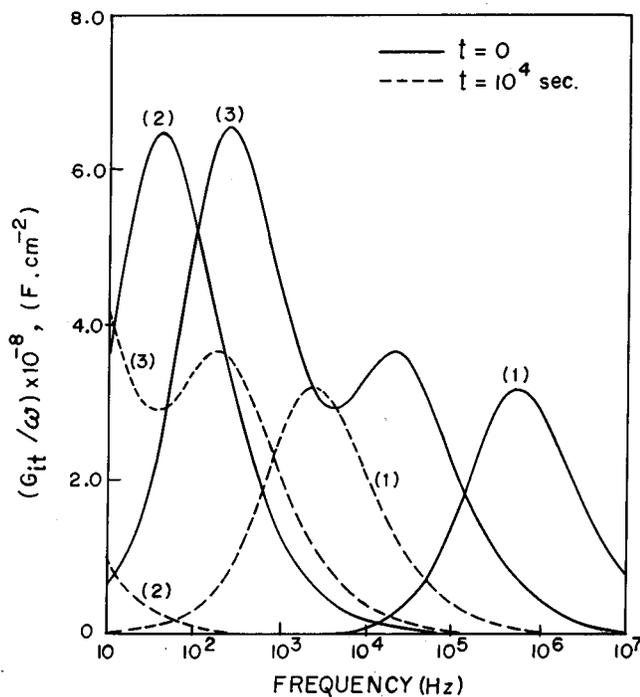
FIG. 10. The  $G_{it}/\omega$  vs  $\omega$  plot of MIS tunnel contact in the presence of interface reaction. Parameters:  $\sigma_a = 10^{-12} \text{ cm}^2$ ,  $\sigma_d = 10^{-14} \text{ cm}^2$ , and  $v_{th} = 10^7 \text{ cm s}^{-1}$ . The values of other parameters including the parameters for curves (1,1), (2,2), and (3,3) are same as those in Fig. 2. The dashed line plots represent variation after aging for time  $t = 10^{-4} \text{ s}$ .
