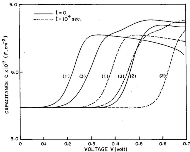
FIG. 8. The capacitance–voltage characteristics of a MIS tunnel device as a function of bias voltage in the presence of interface states and interface reaction. Parameters:  $\sigma_a = 10^{-12} \text{ cm}^2$ ,  $\sigma_d = 10^{-14} \text{ cm}^2$ , and  $v_{th} = 10^7 \text{ cm s}^{-1}$ . The values of the other parameters including those for curves (1,1), (2,2), and (3,3) are same as those in Fig. 2. The variations after a time  $t = 10^4 \text{ s}$  are shown by broken lines.
