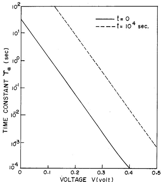
FIG. 5. Variation of time constant  $\tau_a$  of acceptor-like interface states as a function of applied voltage in the presence of interface reaction. Parameters:  $\sigma_a=10^{-12} \text{ cm}^2$ ,  $v_{th}=10^7 \text{ cm s}^{-1}$ , and  $D_{it}^a=5 \times 10^{11} \text{ cm}^{-2} \text{ eV}^{-1}$ . The values of the other parameters are same as those in Fig. 2. The Nature of variation after aging time  $t=10^4 \text{ s}$  is shown by broken line.
