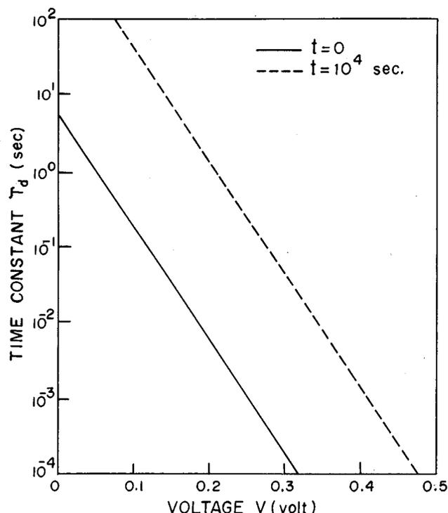
FIG. 4. Variation of time constant  $\tau_d$  of donor-like interface states as a function of applied voltage in the presence of interface reaction. Parameters:  $\sigma_d=10^{-13} \text{ cm}^2$ ,  $v_{th}=10^7 \text{ cm s}^{-1}$ , and  $D_{it}^d=5 \times 10^{11} \text{ cm}^{-2} \text{ eV}^{-1}$ . The values of the other parameters are same as those in Fig. 2. The nature of variation after aging time  $t=10^4 \text{ s}$  is shown by broken line.
