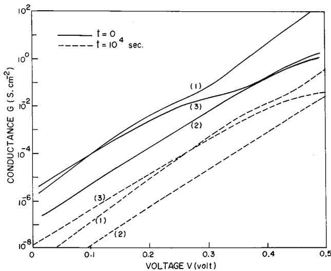
FIG. 6. The variation of ac conductance of a MIS tunnel device as a function of bias voltage in the presence of interface states and interface reaction. Parameters:  $\sigma_a = 10^{-12} \text{ cm}^2$ ,  $\sigma_d = 10^{-14} \text{ cm}^2$ , and  $v_{th} = 10^7 \text{ cm s}^{-1}$ . The values of the other parameters including those for curves (1,1), (2,2), and (3,3) are same as those in Fig. 2. The variation after a time  $t = 10^4 \text{ s}$  of the aging device is shown by broken line curves.
