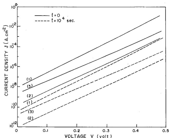
FIG. 3. Current-voltage characteristics of a MIS tunnel contact in the presence of interface states and the interface reaction. Parameters:  $\phi^{1/2}\delta=2$ ,  $A=120 \text{ A cm}^{-2} \text{ K}^{-2}$ , and  $T=300 \text{ K}$ . The values of the other parameters including those for curves (1,1), (2,2), and (3,3) are same as in Fig. 2.
