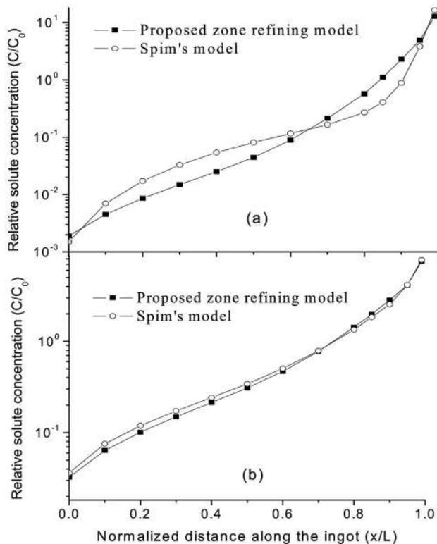
FIG. 5. Comparison of the proposed model with the model of Spim *et al.* (Ref. 13) for (a)  $k=0.4$  after 10 passes (b)  $k=0.8$  after 20 passes.
