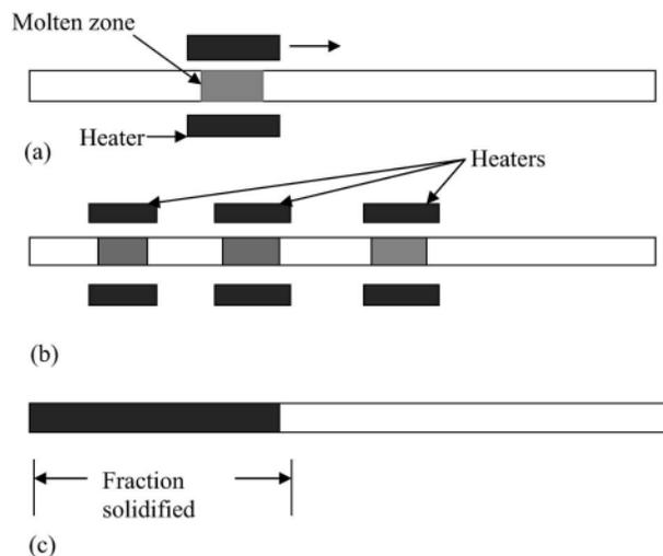
FIG. 1. Schematic sketch of zone melting operation for (a) single pass zone refining, (b) multipass zone refining, and (c) normal freezing.
