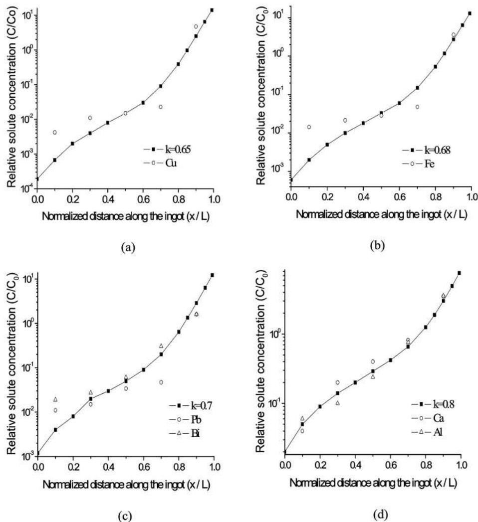
FIG. 7. Comparison of concentration distribution of (a) copper (b) iron (c) lead and bismuth, and (e) aluminum and calcium with the theoretical distribution after 50 passes.
