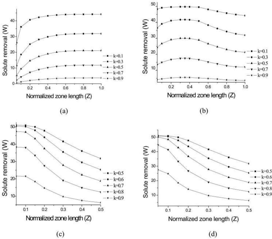
FIG. 2. Effect of the zone length on solute removal after (a) single refining pass, (b) second pass, (c) 30 passes, and (d) 50 passes, with the previous passes operated by effective the zone length that led to maximum solute removal.
