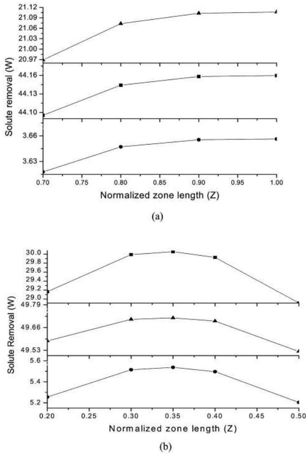
FIG. 3. Enlarged portion for  $k=0.5$ , 0.1, and 0.9 (respectively from top to bottom) of Figs. 2(a) and 2(b) to clearly distinguish the effect of normalized molten zone length upon solute removal.
