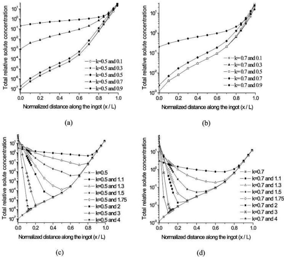
FIG. 6. Effect on impurity concentration profiles having  $k < 1$  along the ingot after 50 passes (a) on the impurity having  $k=0.5$ , (b) on the impurity having  $k=0.7$ , and the same for  $k > 1$ , (c) on the impurity having  $k=0.5$ , and (d) on the impurity having  $k=0.7$ .
