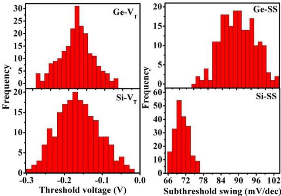
FIG. 3. Histograms for threshold voltage and subthreshold swing due to RDD for  $L_g = 20$  nm,  $W_{fin} = 8$  nm,  $H_{fin} = 15$  nm,  $N_D = 1 \times 10^{19} \text{ cm}^{-3}$ , and  $D_{it} = 1 \times 10^{11} \text{ cm}^{-2} \text{ eV}^{-1}$  at  $V_{DS} = 1.0$  V.
