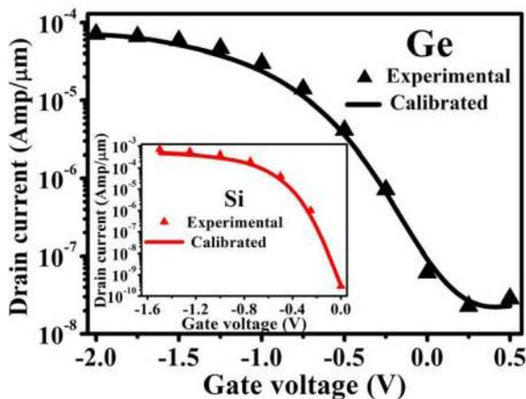
FIG. 2. Calibration of the model for Ge JL FinFET against the experimental data in Ref. 9. Inset shows the calibration of Si JL FinFET with the experimental data in Ref. 15.
