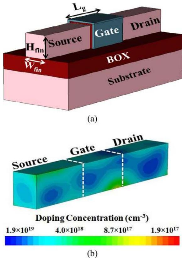
FIG. 1. (a) Schematic device structure and (b) randomized doping profile for JL FinFET.
