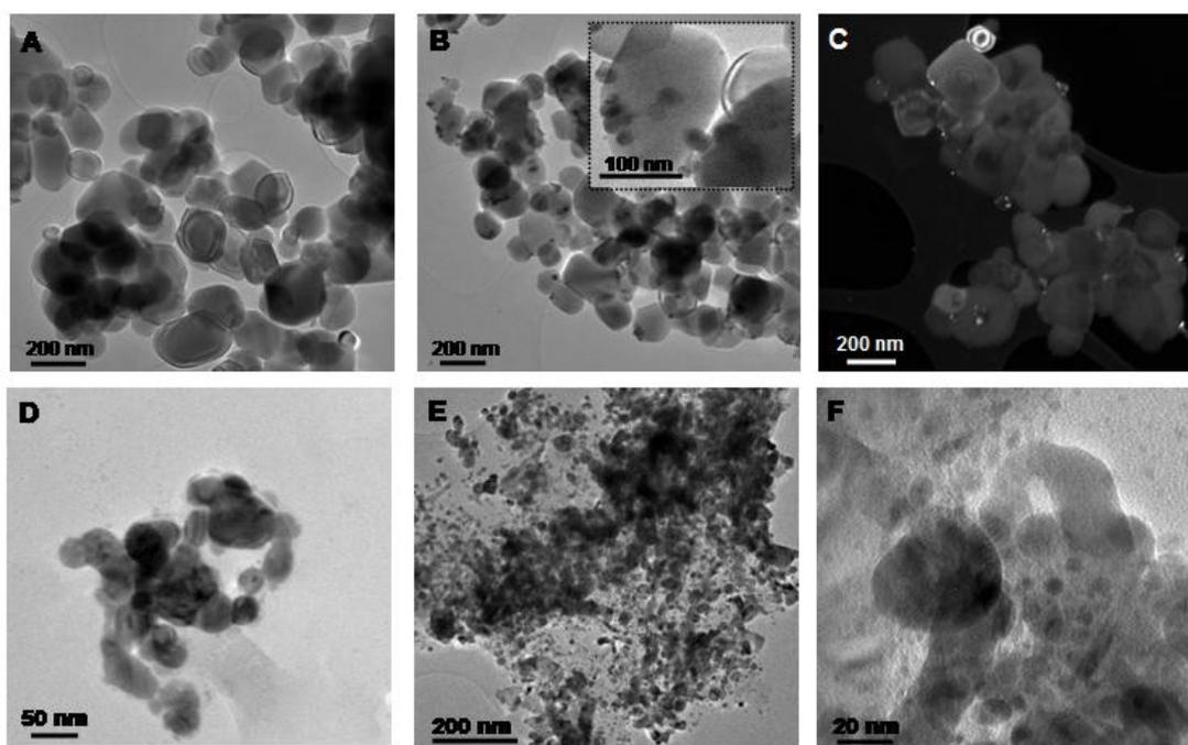
**Figure 2.** (A) TEM image of pristine titania nanoparticles. (B, C) TEM images of Ag nanoparticles on titania surface. (D) TEM image of pristine alumina particles. (E, F) TEM images of Ag nanoparticles on alumina surface.
