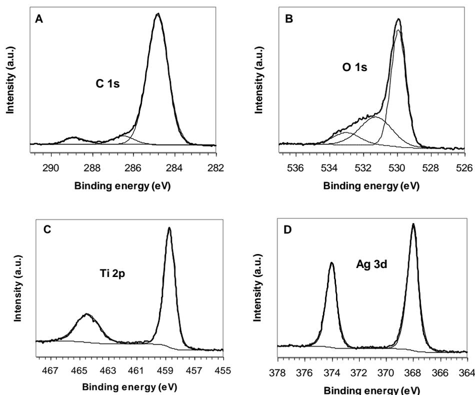
**Figure 3.** (A) C 1s, (B) O 1s, (C) Ti 2p, (D) Ag 3d X-ray photoelectron spectra obtained for TiO<sub>2</sub>-Ag composite nanoparticles.
