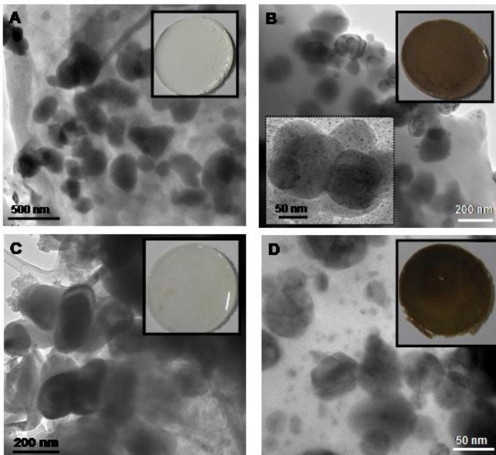
**Figure 8.** (A) TEM image of TiO<sub>2</sub>/epoxy nanocomposite. (B) TEM image of TiO<sub>2</sub>-Ag/epoxy nanocomposite. Inset, bottom left: Ag nanoparticles present on titania surface within epoxy matrix. (C) TEM image of Al<sub>2</sub>O<sub>3</sub>/epoxy nanocomposite. (D) TEM image of Al<sub>2</sub>O<sub>3</sub>-Ag/epoxy nanocomposite. For each epoxy nanocomposite formulated, a specimen of the cured formulation is shown inset.
