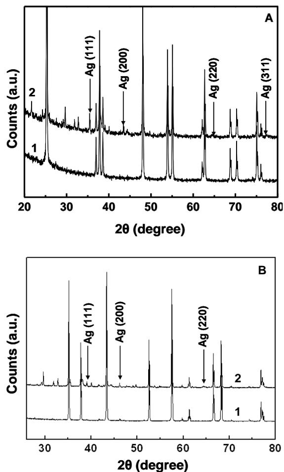
**Figure 1.** (A) XRD pattern of pristine titania (Curve 1) and  $\text{TiO}_2$ -Ag composite nanoparticles (Curve 2). The peaks attributed to Ag nanoparticles are in agreement with fcc crystal structure; (B) XRD pattern of pristine alumina (Curve 1) and  $\text{Al}_2\text{O}_3$ -Ag composite nanoparticles (Curve 2). The Ag peaks and the corresponding planes are arrowed.
