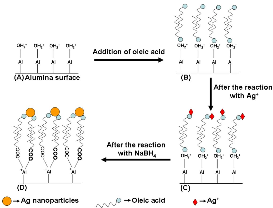
**Scheme 2.** Mode of assembly of  $\text{Al}_2\text{O}_3\text{-Ag}$  composite nanoparticles. The role of oleic acid in the synthesis is indicated.
