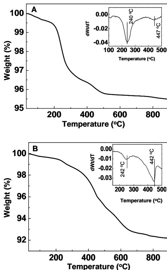
**Figure 7.** (A) TGA trace of  $\text{TiO}_2\text{-Ag}$  composite nanoparticles. Inset: derivative curve, showing maximum mass loss at 240  $^{\circ}\text{C}$ . (B) TGA trace of  $\text{Al}_2\text{O}_3\text{-Ag}$  composite nanoparticles. Inset: derivative curve, showing maximum mass loss at 442  $^{\circ}\text{C}$ .
