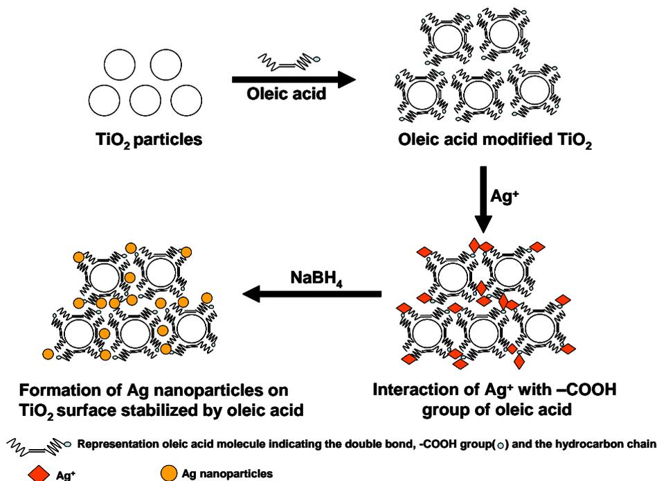
**Scheme 1.** Mode of assembly of  $\text{TiO}_2$ -Ag composite nanoparticles. The role of oleic acid in the synthesis is indicated.
