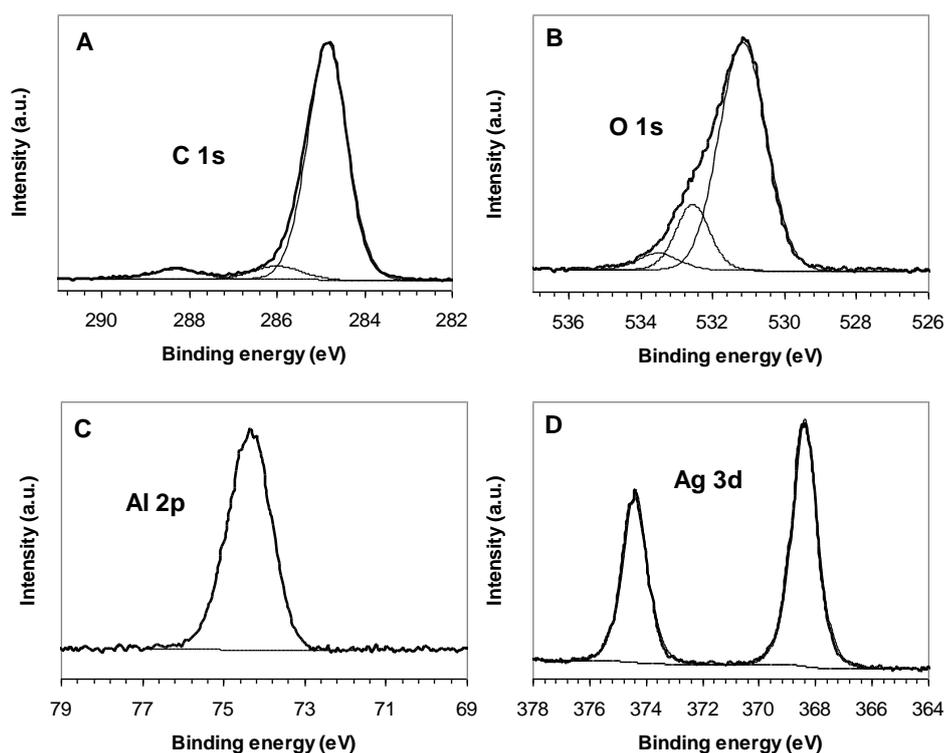
**Figure 5.** (A) C1s, (B) O1s, (C) Al2p and (D) Ag3d X-ray photoelectron spectra obtained for Al<sub>2</sub>O<sub>3</sub>-Ag composites.
