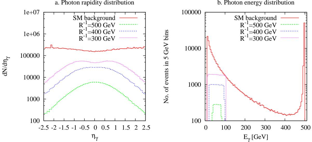
Figure 8: Photon (a) rapidity distribution and (b) energy distribution for  $\gamma + \cancel{E}$  events for signal (dotted, dashed, long dashed histogram) and background (solid histogram) at  $\sqrt{s} = 1$  TeV,  $\mathcal{L} = 500 \text{ fb}^{-1}$  and beam polarization  $(P_-, P_+) = (0.8, -0.6)$ .
