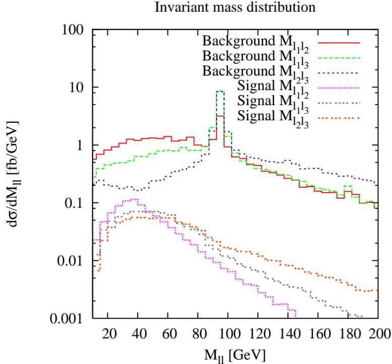
Figure 4: Invariant mass distribution of signal (for  $R^{-1} = 500$  GeV) and background (for  $3\text{-lepton} + \cancel{p}_T$  signal).
