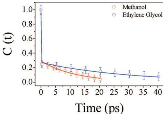
**Figure 6.** Solvation correlation function,  $C(t)$ , of curcumin in methanol and ethylene glycol obtained from fluorescence upconversion experiments. Solvation correlation function is fitted with biexponential decay function. Both the solvents showed the same initial fast component of 50 fs but a different slow component of 12 ps (methanol) and 30 ps (ethylene glycol).
