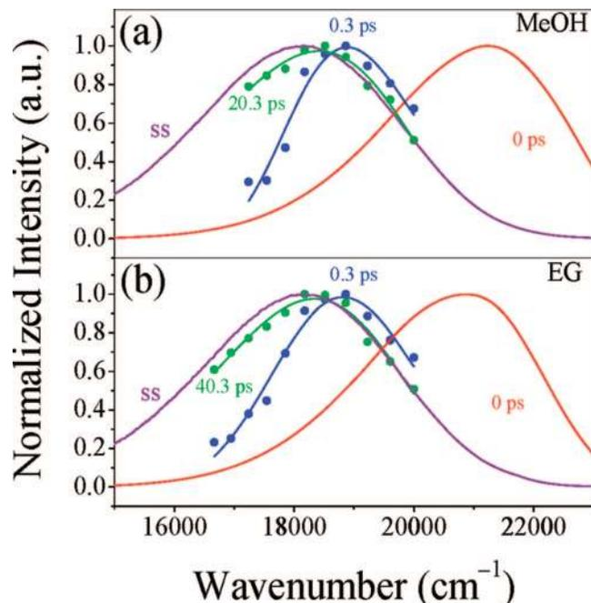
**Figure 5.** Normalized time-resolved emission spectra of curcumin in methanol (MeOH) and ethylene glycol (EG). Steady-state (ss) and “zero-time” ( $t = 0$  ps) spectra are included. Almost 70% of the solvation is complete in both systems within the time resolution of our instrument (300 fs).
