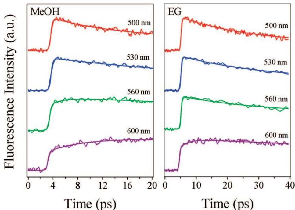
**Figure 4.** Representative normalized wavelength resolved fluorescence upconversion traces of curcumin in methanol (MeOH) and ethylene glycol (EG). Time-resolved emission spectra were constructed by collecting upconversion traces over a range from 500 to 600 nm at intervals of 10 nm. The time-resolved traces at the red end (600 nm) show a growing component, which is the signature of solvation dynamics.
