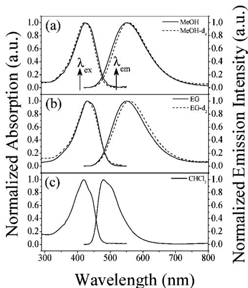
**Figure 2.** Normalized absorption and fluorescence spectra of curcumin in (a) methanol (MeOH), deuterated methanol (MeOH- $d_4$ ), (b) ethylene glycol (EG), deuterated ethylene glycol (EG- $d_2$ ), and (c) chloroform (CHCl $_3$ ).
