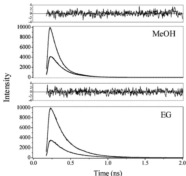
**Figure 7.** Polarized fluorescence traces and residuals of fits for curcumin in methanol (MeOH) and ethylene glycol (EG). Fitting parameters are given in Table 3. The upper trace represents that emission is collected parallel ( $I_{\parallel}$ ) and the lower trace is collected perpendicular ( $I_{\perp}$ ) to the excitation polarization.  $\lambda_{\text{ex}} = 407$  nm,  $\lambda_{\text{em}} \geq 500$  nm.
