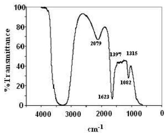
**Figure 8.** Infrared spectra of partially degraded DEA.
