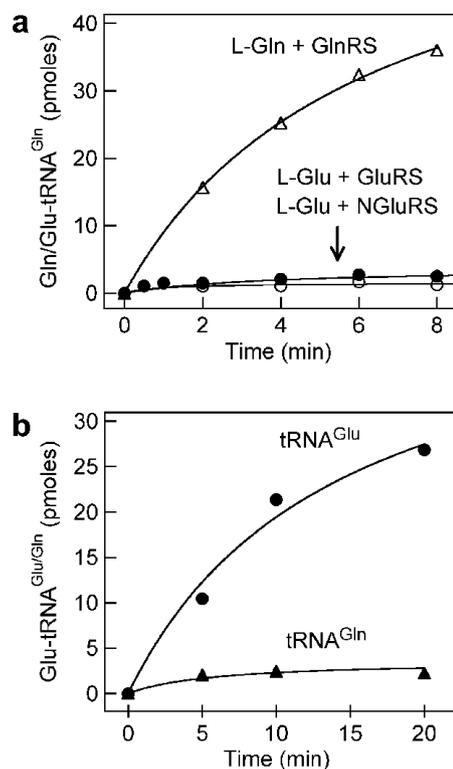
**Fig. 4.** (a) Non-cognate aminoacylation (glutamylation) assay curves of  $EctRNA^{Gln}$  with *EcGluRS* (3 ng/assay point) (●) and *NGluRS* (1.5  $\mu$ g/assay point) (○). For comparison cognate aminoacylation (glutaminylation) assay curve of  $tRNA^{Gln}$  with *EcGlnRS* (1 ng/20  $\mu$ l assay point) ( $\Delta$ ) is also shown. (b) Glutamylation assay curves of cognate ( $tRNA^{Glu}$ ; ●) and non-cognate ( $tRNA^{Gln}$ ; ▲) tRNA by *cGluGlnRS* (1  $\mu$ g/assay point).
