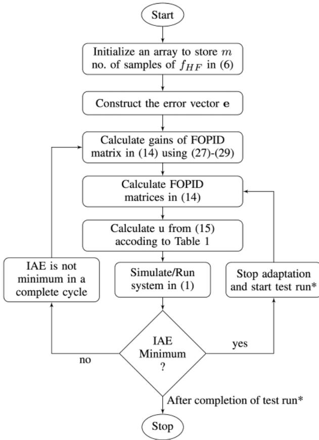
**Fig. 2** Flowchart representation of the adaptive FOPID controller in the HF domain
