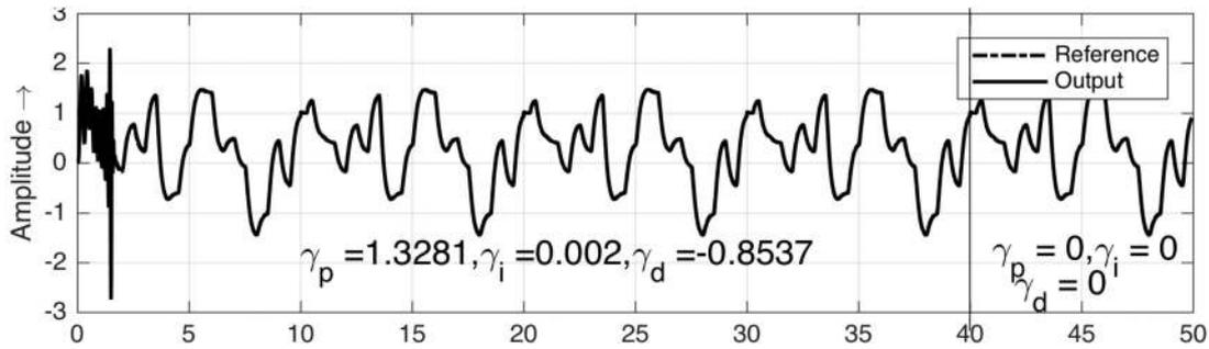
Fig. 7 Performance characteristics of the non-linear DC motor of case study 2 using the HFAFOPID controller
