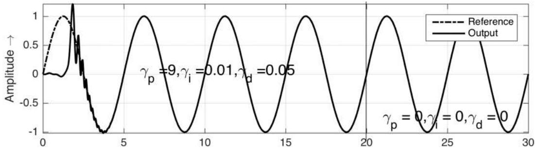
Fig. 4 Performance characteristics of the Duffing's system with disturbance using the HFAFOPID controller
