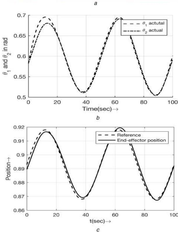
**Fig. 9** (a) Real-life PC-based experimental arrangement for the two-link manipulator; (b) Performance characteristics of the joint-angles of two-link manipulator defined (33) with the HFAFOPID controller when the frequency of the reference signal is 0.02 Hz; (c) Performance characteristics of the position of the end-effector of two-link manipulator defined (33) with the HFAFOPID controller when the frequency of the reference signal is 0.02 Hz
