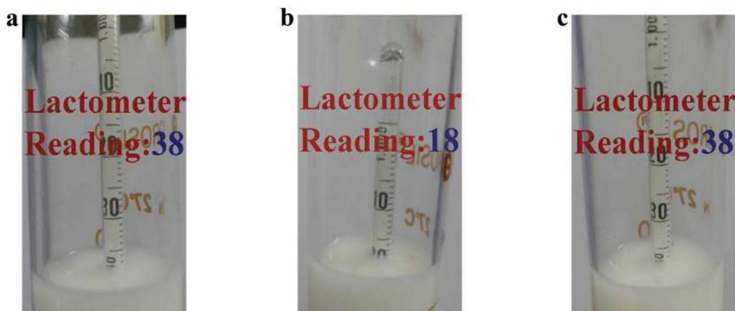
**Figure 9.** Lactometer readings of local milk (a) before and (b) after dilution with water. Panel c shows the local milk after adulteration with sugar.
