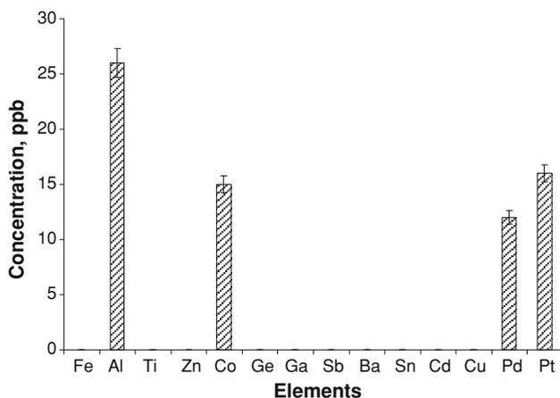
**Fig. 2** Different elemental impurities in the MilliQ fraction containing <sup>68</sup>Ga eluted from the anion exchange resin
