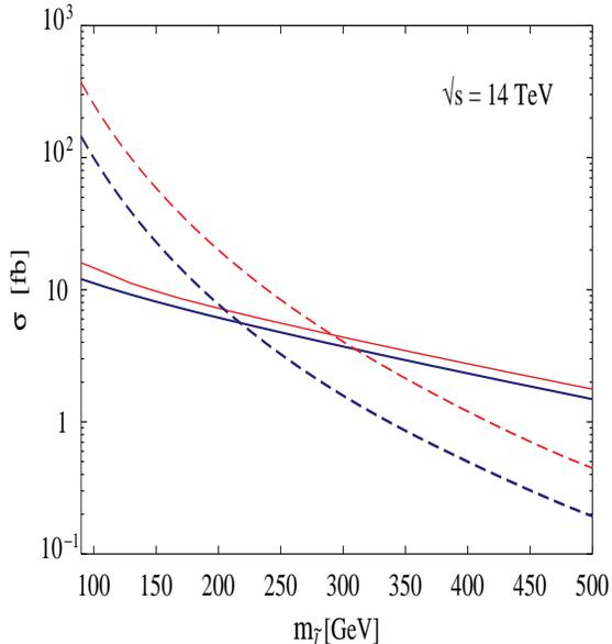
Figure 2: *The total cross section (solid lines) for slepton pair-production at the LHC in association with two forward jets. The cuts of eqns.(1a–1c) have been imposed on the VBF rates. The CTEQ4L parton distributions have been used with the factorization scale set at  $m_{\tilde{l}}$ . The dashed curves represent the corresponding DY cross sections. In each case, the upper and lower curves correspond to  $\tilde{\ell}_L$  and  $\tilde{\ell}_R$  (one flavour) respectively.*
