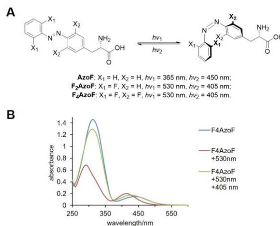
**Figure 1.** A) Photoisomerization of azobenzene analogs **AzoF**, **F<sub>2</sub>AzoF**, and **F<sub>4</sub>AzoF**. B) UV/Vis spectra of the *trans*-photoisomer (>99% *trans*, blue, in the dark-adapted state), *cis*-photoisomer (91% *cis*, red, 530 nm), and *trans*-photoisomer (84% *trans*, green, 405 nm) of **F<sub>4</sub>AzoF** in PBS (pH 7.4).
